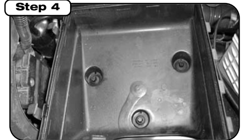
Remove lower half of filter box, unscrew 3 inserts and transfer inserts to new filter housing.
