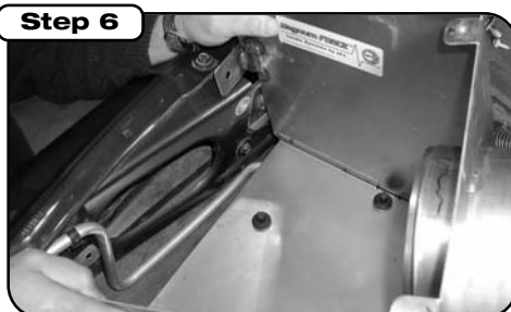
Lower housing into place, tab for ground screw tucks behind A/C line first, then lower to clear turbo housing. Housing should clear A/C line, line up rubber mounts and secure by pushing down hard or screwing mounts in. Install fender brace screw and ground screw and wire.
