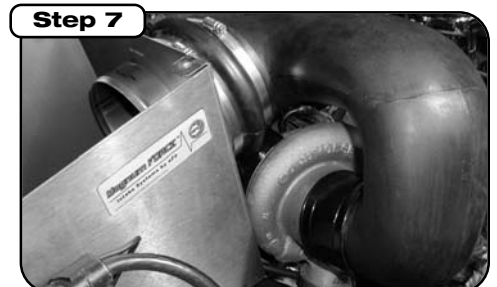
Slip boots over intake tube and install on turbo and filter housing. It may be easier to install clamps after tube is in position. If filter restriction gauge is desired, drill an 11/16 hole with a woodworking spade bit and transfer grommet and sensor to new intake tube. Sensor should be placed near larger end of tube for accurate results.
