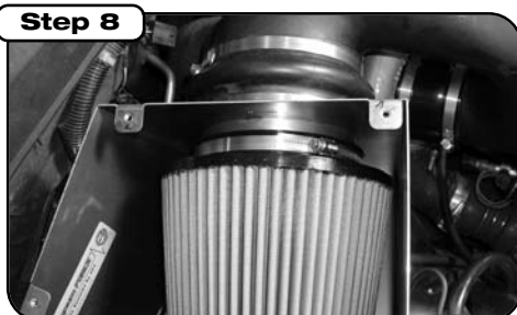
Install factory pre-oiled filter into housing. Install cover and make a final check for loose clamps, pinched wires etc. before starting engine.
