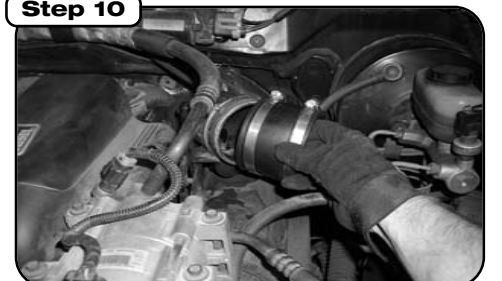
Place provided clamps loosely over provided coupler and place onto factory turbo inlet elbow
