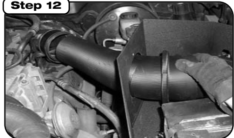
insert tube through heat shield so that the flange is on the inside of the heat shield and insert into coupler installed in previous step.
