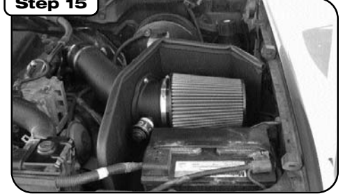
Complete kit installed.
