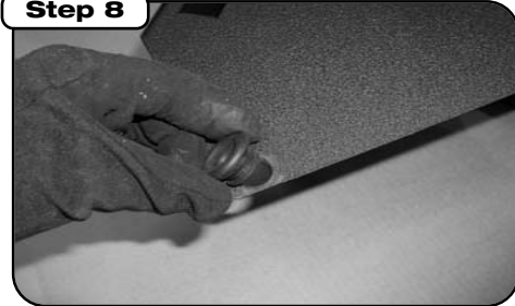
Place saved grommets into holes on the bottom of the aFe heat shield.
