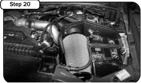
Step 20 Your installation is now complete. Make sure you tighten all clamps and check all electrical connections. Re-check periodically.
