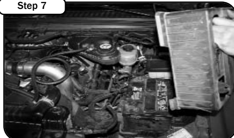
Step 7 Disconnect passenger side battery terminals, remove battery cover and battery from engine compartment.
