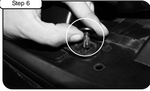
Remove plastic clip. Repeat steps 4-6 for remaining clip. (Save for later installation)
