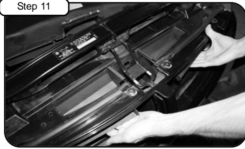
For easier installation, the next three steps will require an assistant. Have person A hold the scoops in position as shown.
