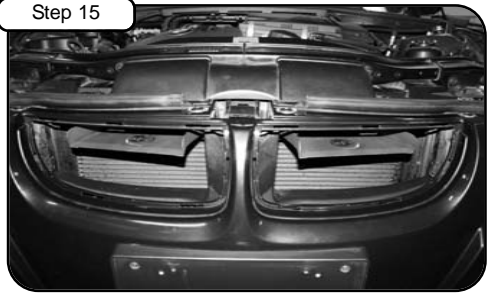
Your completed D.A.S. installation will look like this. Check and make sure they are secure. Re-install grills by lining up tabs and pushing them in until they snap into place. Thank you for choosing aFe!
