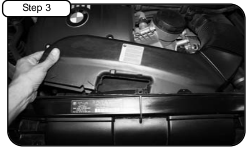
Pull back ram air duct and remove.
