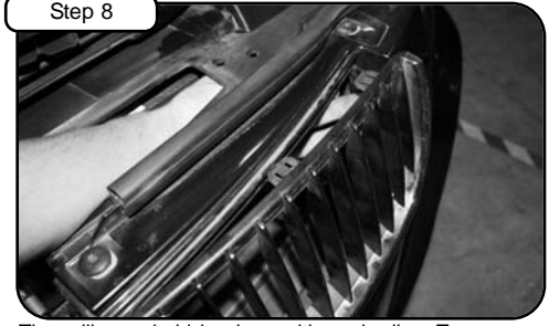
The grills are held in place with push clips. To remove, reach in behind each grill and push forward.
