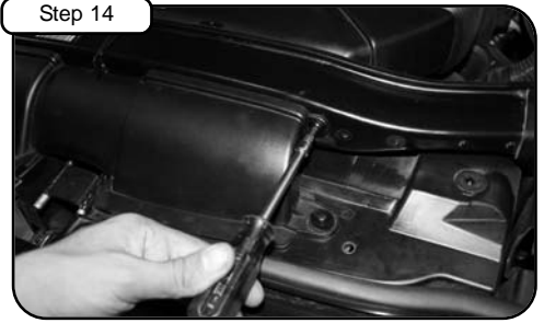
Re-position ram air duct from step 3. Secure using the 2 screws from step 2 and tighten using T25 torx bit.
