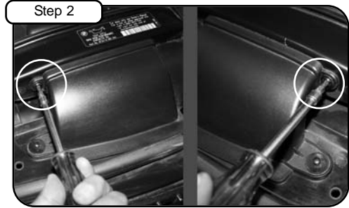
Remove screws on ram air duct using T25 torx bit. (Save for later installation)
