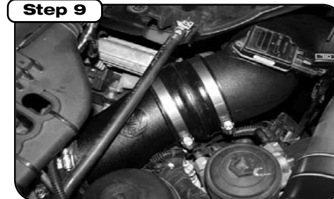
Step 9 Slide tube through housing hole and turning tube to fit through. Do not attach tube to housing until Step 10. (Install MAF sensor once tube is through housing)
