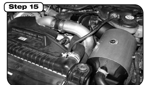
Step 15 Complete intake installed. Make sure all clamps are tight and that all electrical components are secure. Check and retighten connections and filter after a few hours of operation. Reconnect battery terminal. Thank you for choosing aFe!
