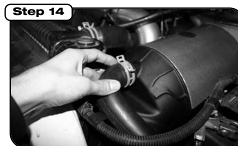
Step 14 Remove factory auxiliary air tube from stock intake track and install onto aFe housing. Re-route hose under battery terminal and towards inner fender wall.
