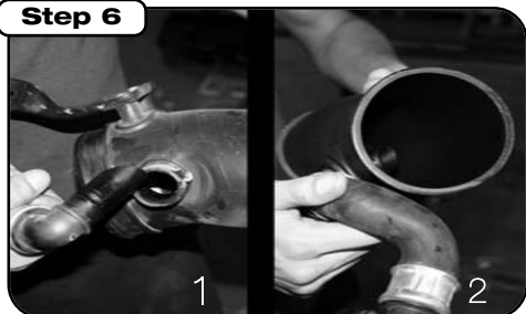
Step 6 Using a 10mm socket or wrench remove tube support bracket from engine. Loosen clamp at turbo with a 5/16 nut driver or screwdriver. 1. Remove crank case breather from factory tube. 2. Place rubber grommet into with 1" opening hole and press crank case breather into grommet on new tube.
