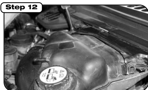
Step 12 Attach tube to urethane coupler at aFe turbo inlet with provided clamp. Then use provided 1/4 20" hardware and bolt housing to tube. Reinstall radiator overflow reservoir and reconnect 1/2" hose.
