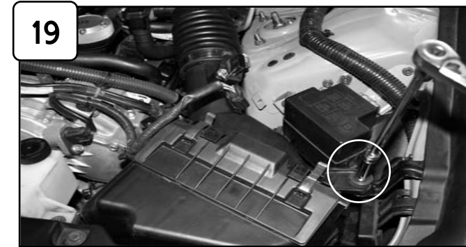
With 10mm socket or wrench, loosen the bolt holding in air box.
