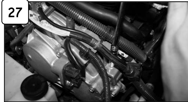
Loosen bolt on engine securing harness bracket.
