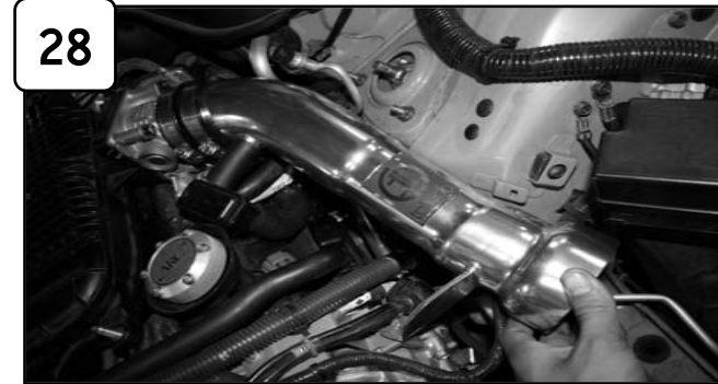
First re-connect MAF sensor harness. Install into vehicle and position. Do not tighten clamps.
