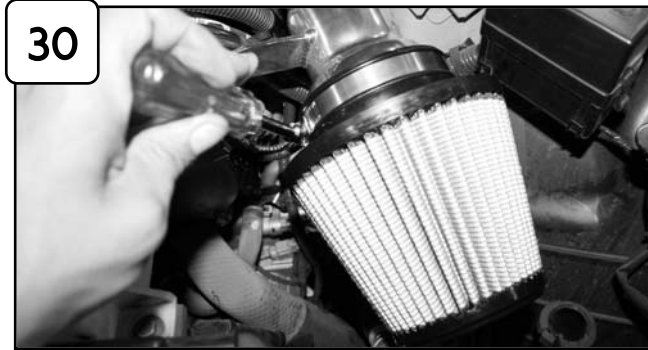
Tighten all clamps using 5/16" nut driver. Install air filter and tighten using 5/16" nut driver.
