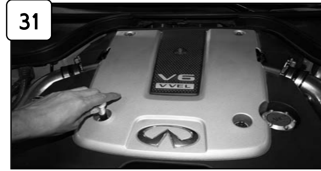
Re-install engine cover and tighten using 10mm socket or wrench.
