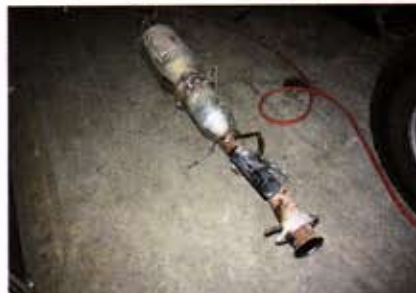
With the factory diesel particulate filter and catalytic converter removed from the truck, you can plainly see just how large and restrictive these units can be.
