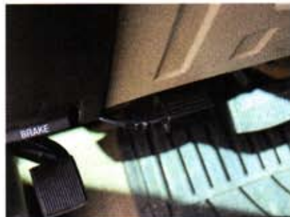
The Black Maxx tuner installed in just 30 minutes, with just one wire to tap into for power to the monitor and this OBD-II connector, it's a pretty straight forward and easy installation.
