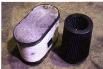
While the AFE filter looks smaller, it flows much better and doesn't require replacing, just rinse it out, re-oil it, and clamp it back in.
