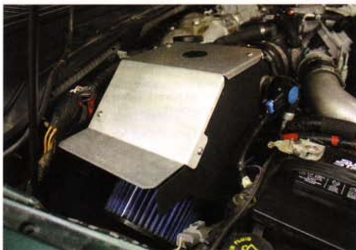
The AFE Stage II cold air intake not only offers easy breathing for the sequential turbochargers, it offers effective filtering through a five-layer reusable cleanable filter. Installation took just 30 minutes with basic hand tools.
