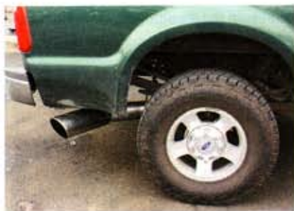
The new 5-inch downpipe back exhaust system, complete with a 6-inch tip, from H&S Performance really opened the door for some big performance gains and a deep throaty exhaust note.
