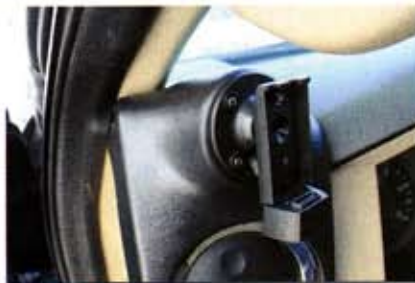
H&S Performance offers this molded dash mount, making for a nice clean install, the wire can be stashed away behind the door molding and down behind the dash, total install of the Black Maxx took less than 30 minutes.
