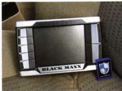
The Black Maxx's color screen monitor is equipped with a small SD card for easy software updates and user adjustable tuning options, such as torque converter lockup speed and transmission shifting strategies.
