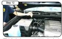
With button head screws provided tighten down housing cover with 5/32" allen key. Re-Install engine cover.
