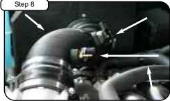
Remove MAF sensor from OE air box using phillps screwdriver. Re-install to new aFe tube with hardware provided (make sure gasket and nylon spacers are between tube and sensor) using flat head screwdriver.Install brass hose fitting.
