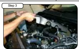
Lift up and remove engine cover.
