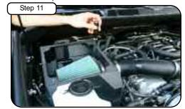
Place air filter into housing and tighten using 5/16" nut driver.
