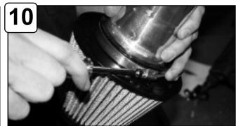
Install air filter to intake tube and tighten using 5/16" nut driver.
