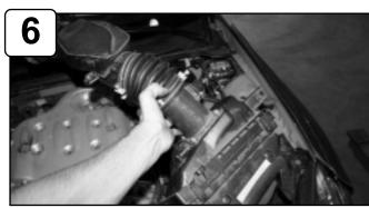
Carefully remove stock air box assembly out of vehicle. (ram scoop optional.)
