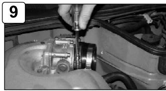
Install coupler with clamps to throttle body. Tighten clamp on throttle body side only.
