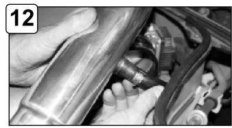
Attach crank case line to intake tube.
