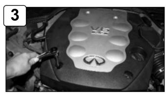
Loosen the 4 bolts using 10mm socket or wrench holding in engine cover and remove.
