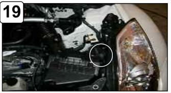
With 10mm socket or wrench, loosen the bolt holding in air box.
