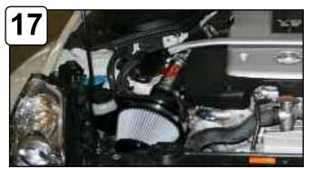
Install trim seal to housing. Nismo, cut trim seal to fit configuration of strut brace. Continue to page 3 for driver side installation..
