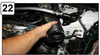
Remove complete intake out of vehicle.
