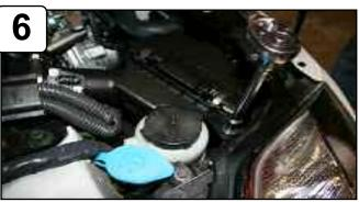
Loosen clamps using 5/16" nut driver. Loosen bolt holding in tube with 10mm socket or wrench. Pull back crank case line from vent box.
