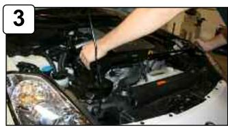
NISMO 350Z only, remove front strut brace before installation.
