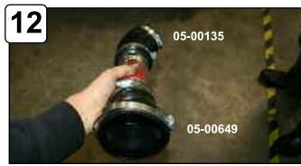
With couplers and clamps provided, attach to tube. Arrow direction on tube points towards throttle body!
