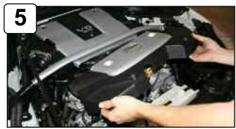
With 10mm socket or wrench, loosen the 5 bolts holding in engine cover and remove.
