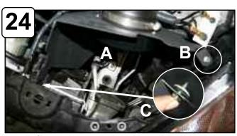
Install filter adaptor to housing using button head screws provided. A)Now install housing into vehicle with bolt on bottom of housing from step 23. B)w/ provided screw and washer install to side of housing. C)Install radiator bracket bolt from step 23 by inserting through housing and using sealing washer.
