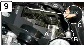
Install filter adaptor to housing using button head screws provided. A)Now install housing into vehicle with screw on bottom of housing from step 4. B)With provided screw and washer install to side of housing. C)Install bolt from step 8 by inserting through housing and using sealing washer.
