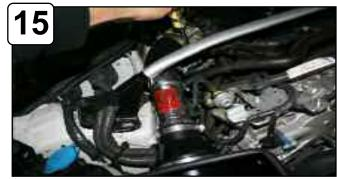
Tighten all clamps using 5/16" nut driver. Re-connect MAF sensor harness.
