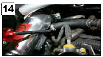
From step 11, install 1/2" plastic fitting into rubber grommet on bottom of tube. *Make sure fitting is inside of tube.*
