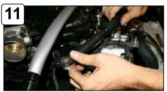
With 6"L 5/8" hose, 1/2" plastic elbow and mini clamp provided tighten at end of hose. On other end with 5/8" straight fitting, connect to stock crankcase line. Make sure 1/2" elbow is facing up under intake tube side. see step 14
