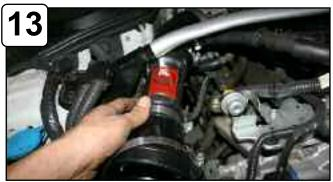
Install into vehicle and position tube. (Elbow coupler on throttle body and reducer coupler on filter adaptor) *Do not tighten clamps.*
