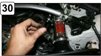
Tighten all clamps using 5/16" nut driver. Re-connect MAF sensor harness.
