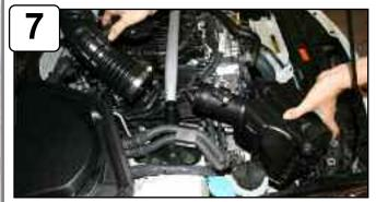
Remove complete intake out of vehicle.
