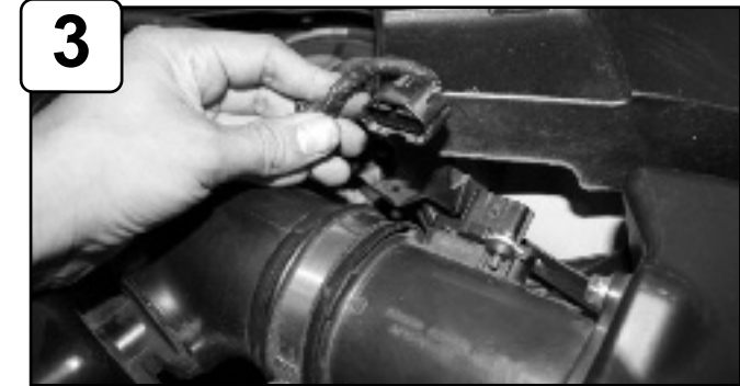
Disconnect MAF sensor harness. Unclip upper half of air box. Loosen clamps using 10mm socket or wrench.
