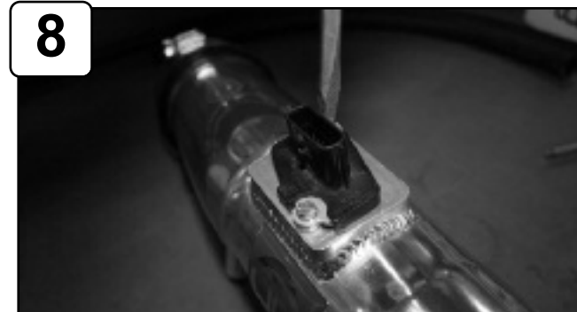
Install MAF sensor to upper tube assembly and secure using provided M4 screws.
