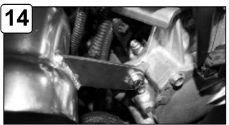
Secure tab to engine and tighten using provided M6 screw and flat washer.
