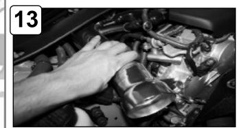
First re-connect MAF sensor harness. Install into vehicle and position tube. *Do not tighten clamps.*
