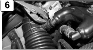
With pliers pull back crank case line from intake.
