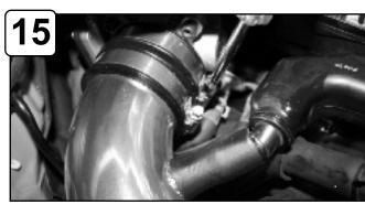
Tighten all clamps using 5/16" nut driver. Attach provided 5/8" hose to intake tube and plenum.
