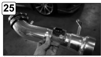
Attach coupling with clamps to tube.
