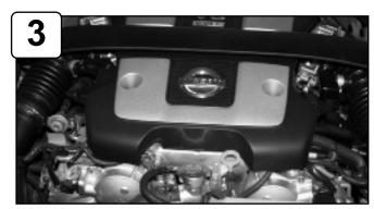
With 10mm socket or wrench, loosen the 2 bolts holding in lower engine cover and remove.
