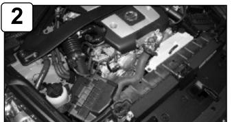
Complete Stock passenger side intake. Please disconnect battery terminals before installation.
