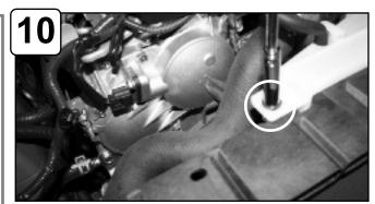
With 10mm socket or wrench loosen the 1 bolt on the radiator resovoir.
