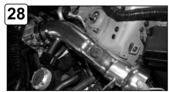
First re-connect MAF sensor harness. Install into vehicle and position. *Do not tighten clamps*.
