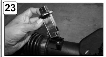
Remove MAF sensor from stock intake.
