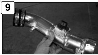
Install MAF sensor to new tube using provided M4 screws. Attach coupling with clamps to tube.
