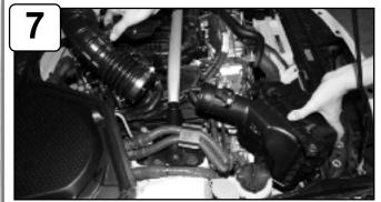
Remove complete intake out of vehicle.
