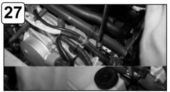
Loosen bolt on engine securing harness bracket.
