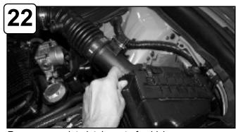
Remove complete intake out of vehicle.
