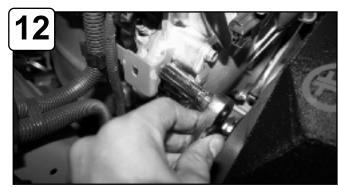
Loosen bolt on engine securing harness bracket.
