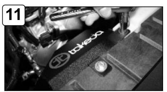
Install housing and secure to radiator support and tighten using bolt from previous step. Secure other tab using provided M6 screw, flat washers and nut.
