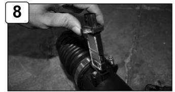
Remove MAF sensor from stock intake.
