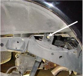
6. Using the stock nuts and bolts, install your new shocks with the top eyelet first and the bottom eyelet second.
