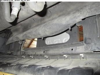
19. Remove 15 of the 8mm bolts to remove the lower lip of the front bumper and pry off lower bumper cover off
