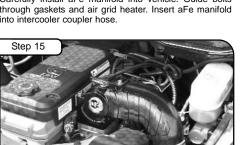
Your installation is now complete. Please check all bolts and screws perodically. Re-tighten if necessary. Thank you for choosing aFe! **Place the included CARB EO sticker** on or near the Charge Air Manifold on a smooth, clean surface. EO identification label is required to pass the Smog Check Inspection.
