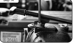
Install the engine oil dipstick using M6 fender washer and socket cap screw provided. Tighten using 5mm allen key (See notes 1, 2 & 3). Attach the engine wire harness to the aFe manifold.
