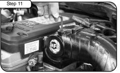
With 6mm hexagonal bit provided and 6mm socket, install the four mounting bolts. Do not tighten completey!
