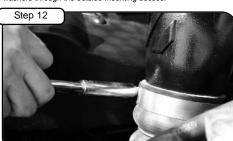
Tighten coupler hose clamp with 11mm socket (See notes 2 & 4). Tighten the four mounting bolts from Step 11 (See notes 2 & 5).
