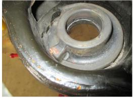
3. Using a screw, or floor jack, raise the lower control arm into position, and align the to the upright. Align bolt, and torque to factory specs using a 18 mm socket, and open wrench.
