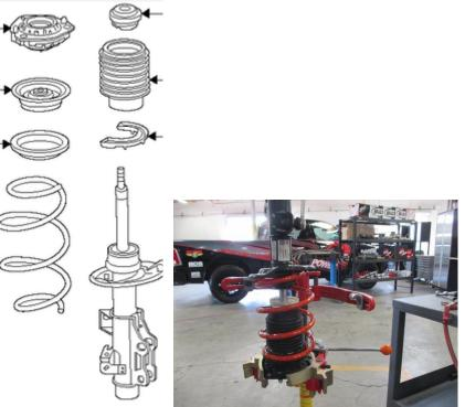
Install the strut assembly into the vehicle by lifting into place, and positioning the upper mount to the body. Note there are 3 studs to pilot into the body. Having a helper on hand, reinstall the (3) upper bolts using a 13 mm socket. Torque to 25 lb-ft.
