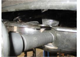
6. Re-attach the end links to the upright and torque to 25 lb-ft.
