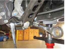
Using a 18 mm wrench and 15 mm socket remove the bolt holding the lower control arm to the upright. Slowly lower the control arm to release tension on the OEM springs, and remove spring from vehicle.
