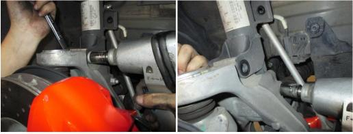
9. Reinstall the sway bar end link, ride height sensor, and reinstall the linkage back on the spindle housing.
