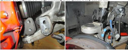
14. Last make sure you remove the top 3 bolts you broke lose earlier so you can remove the strut from the vehicle
