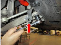
7. Remove the 2 bolts using a 18mm socket and box wrench that hold the strut into the spindle.
