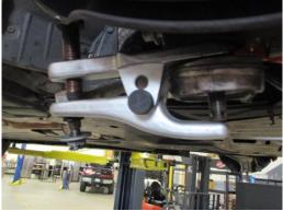
11. Once the lower arm is free. Remove the 2 lower bolts using a 17mm socket that run through the spindle.
