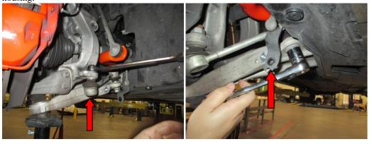
11. Reinstall the brake line bracket onto the spindle and reinstall the strut electronics plug.
