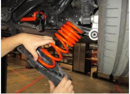
2. Using a screw, or floor jack, raise the lower control arm into position, and align control arm to the upright.
