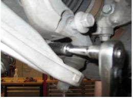
12. Make sure that you have someone to help you hold the spindle. Once the 2 bolts are out the spindle will separate.
