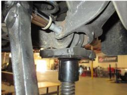
5. Slowly lower the control arm to release tension on the OEM springs, and remove spring from vehicle.
