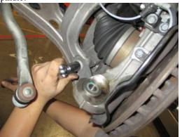
8. Once the lower bolts are tight. Push the spindle up and tighten the 2 strut bolts.
