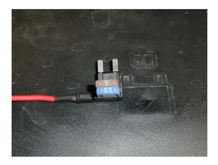
35. Install the fuse removed in Step 34 and insert it into the open location on the supplied adda-harness fuse adapter (not in line with the wire).
