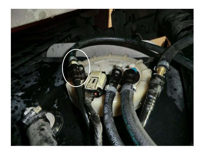
15. Install the supplied fuel return line to the female side of the stock return fuel line (as shown below).
