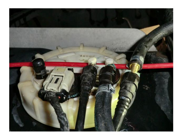
13. Install the supplied fuel outlet hose (with black "AN" fitting) onto the female side of the stock fuel line (shown below).
