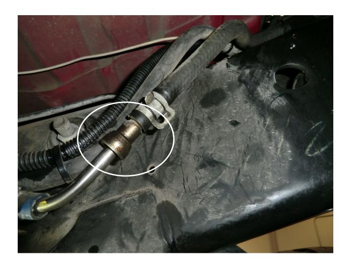
25. Disconnect the stock fuel pump feed hose located on the inside of driver's side frame rail under the driver's door.
