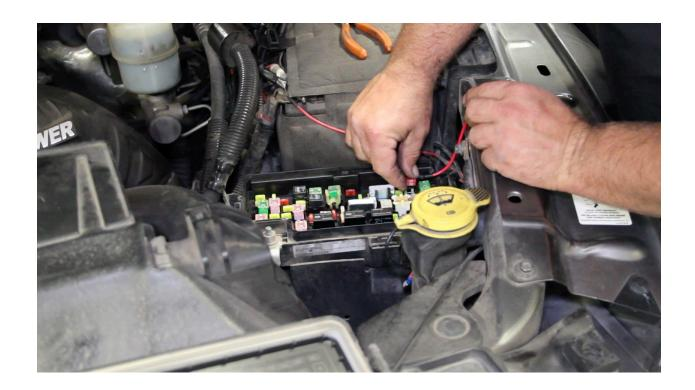
36. Install the add-a-harness fuse adapter (with installed fuses) into the 12-volt ignition source inside the fuse box.
