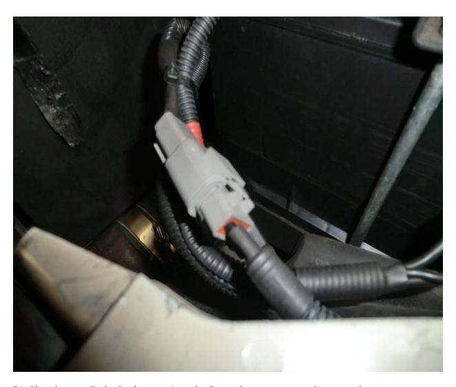
31. Plug the supplied relay harness into the Deutsch connector on the power harness.
