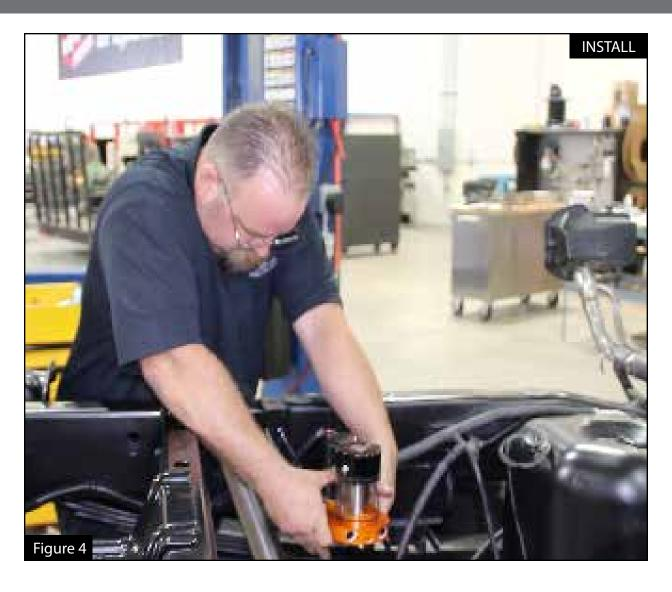
Step 4: Install the bracket onto the frame.
