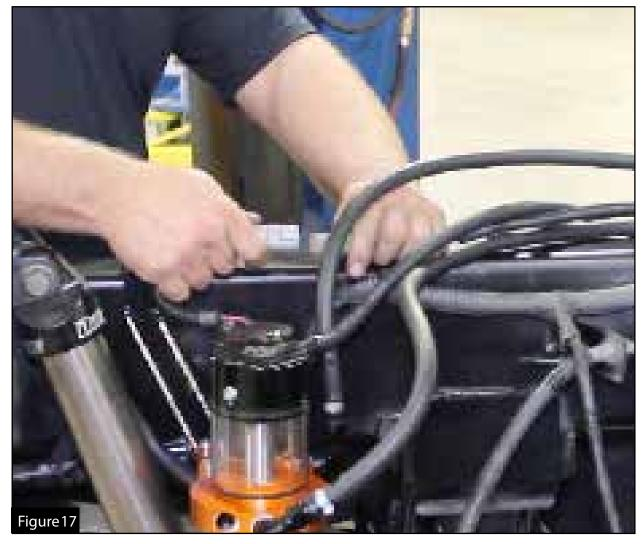
Step 21: Route the supplied wiring harness along the frame.
