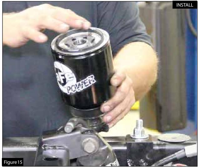
Step 19: Attach supplied water seperator bowl onto the supplied fuel filter. Using a light oil, lube the gasket on the fuel filter before installation.
