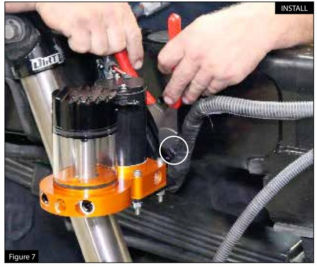
Step 7: The mounting tab located on the stock wire harness, needs to be cut off. (Location shown above)
