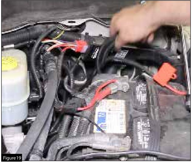
Step 24: Run the remaining wire harness along the frame to the engine compartment. Secure using supplied zip ties.
