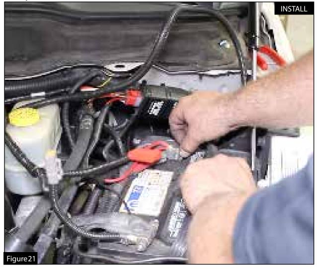
Step 26: Connect the red wire ring terminal to the positive side of the battery.
