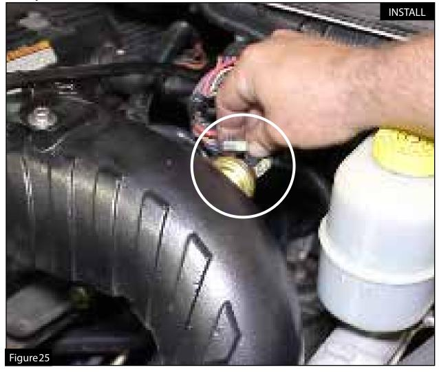
Step 30: Plug the wire loom into the connections on the pressure sensor.
