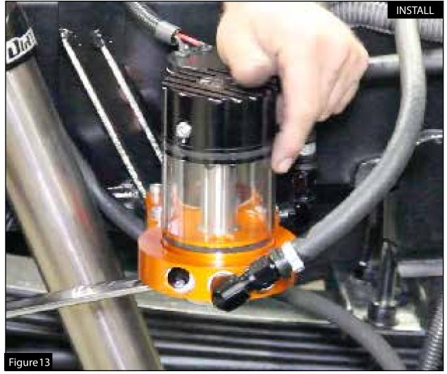
Step 14: Turn sight glass to the desired angle and using a 1-1/4" wrench, tighten the center nut under the DFS780 manifold.
