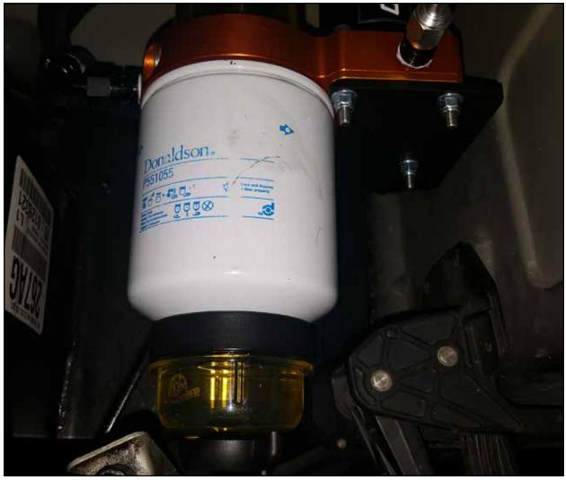
Step 6: Using a light oil, lube the gasket on the supplied fuel filter and install on the fuel manifold assembly. Thread the supplied water separator bowl onto the fuel filter.
