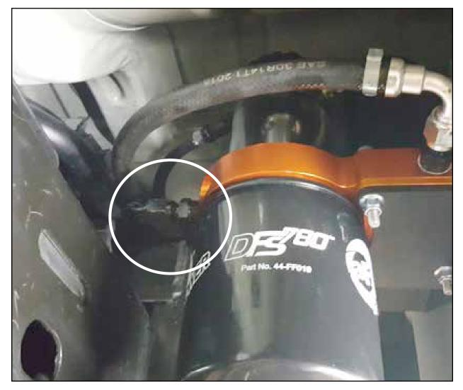
Step 19: Install the fuel outlet hose (black  $90^{\circ}$  -6 AN fitting) onto the male -6 AN fitting on the fuel outlet port of the fuel manifold assembly an tighten.
