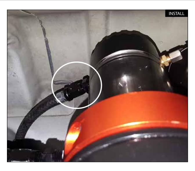
Step 20: Install the fuel return hose (-4 AN fitting) onto male -4 AN fitting on the top of the sight glass cover and tighten.
