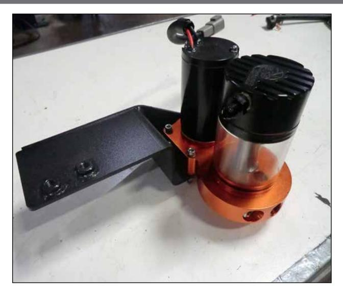
Step 3: Mount the supplied fuel manifold assembly to the carbon steel frame bracket using the supplied hardware and tighten.
