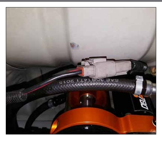
Step 22: Plug the Deutsch connector on the supplied power harness into the mating connector on the fuel pump motor.
