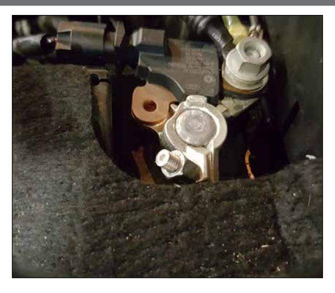
Step 30: Connect the black wire ring terminal on the power harness to the negative side of the battery.
