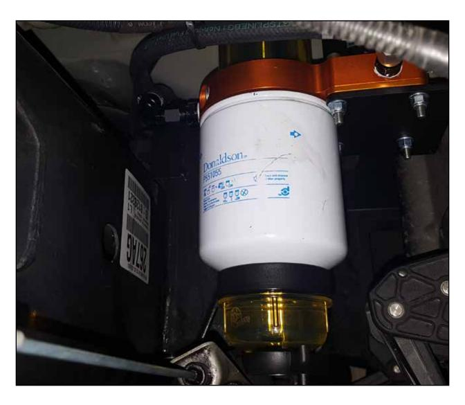
Step 40: Turn the key to the "Run" position and watch to see if the sight glass fills with fuel. If the sight glass does not fill with fuel, use the tank valve (on the top of the sight glass cover) to release any trapped air. If the sight glass still does not fill, try starting the engine.
