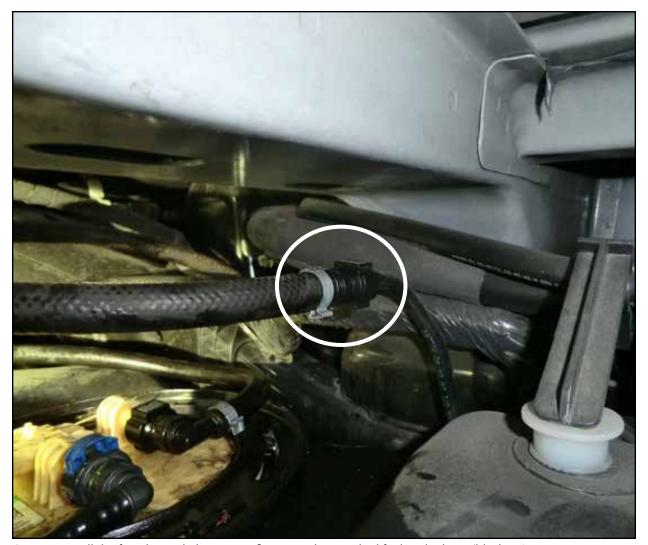
Step 14: Install the female quick disconnect fitting on the supplied fuel outlet hose (black  $90^{\circ}$  -6 AN fitting - shown below) onto the male side of the stock fuel feed line.
