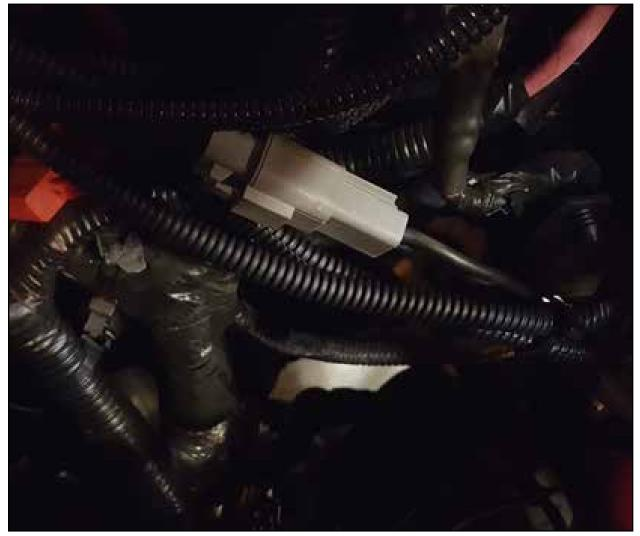
Step 31: Plug the supplied relay harness into the Deutsch connector on the power harness.
