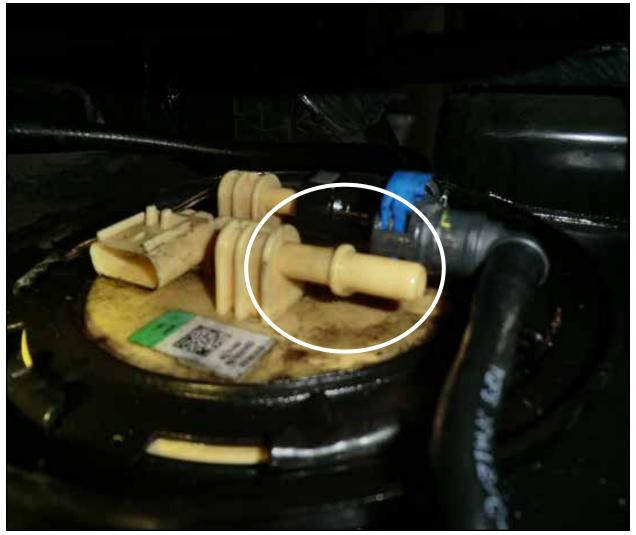
Step 15: Disconnect the factory return fuel line from the return connection on the tank.
