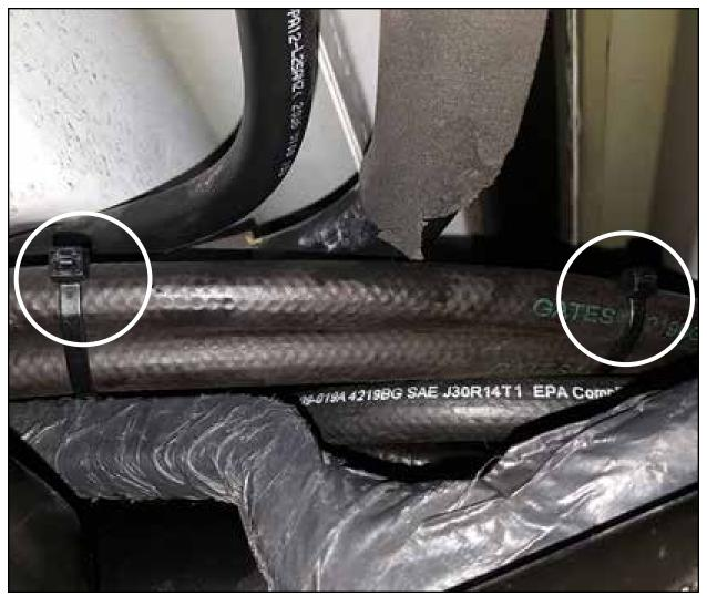
Step 21: Using the supplied nylon cable ties, secure the new hoses (as shown above).
