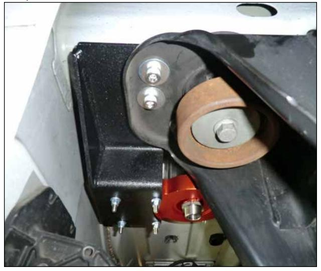
Step 4: Mount the carbon steel frame bracket and the supplied fuel manifold assembly to the frame using the supplied hardware and tighten.
