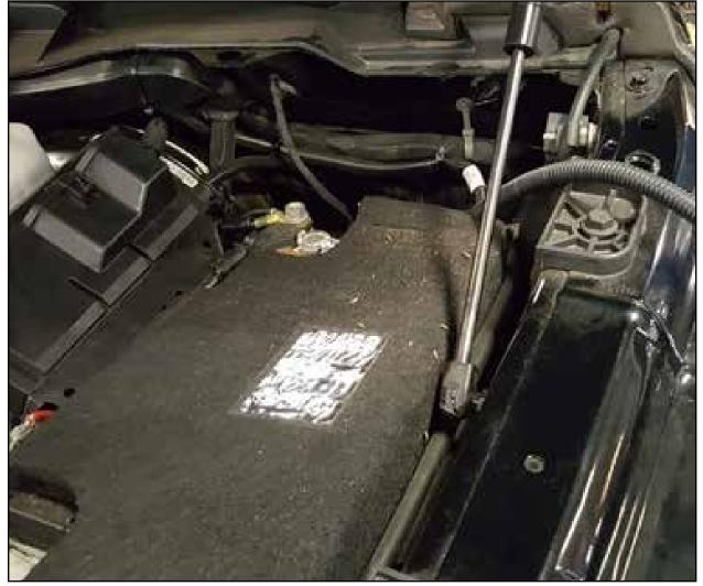
Step 27: Run the other end of the power harness along the frame into the engine compartment.
