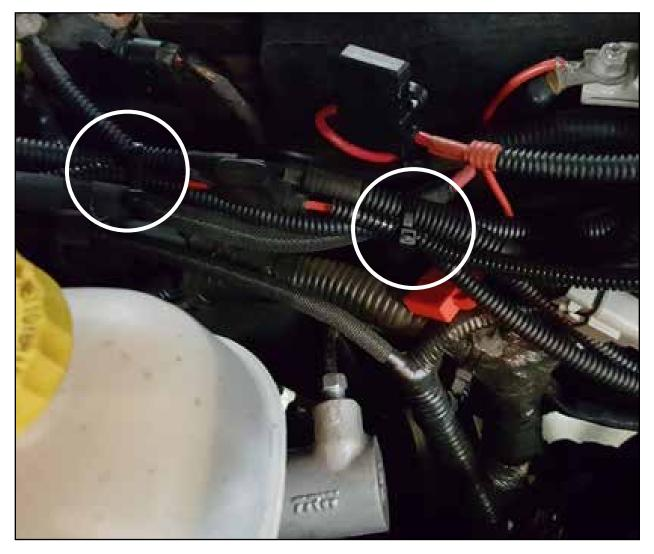
Step 38: Carefully route the power wire outside the fuse box and reinstall the cover (making sure not to pinch the wire).
