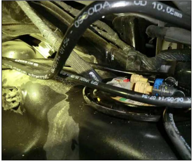
Step 10: Clean the area around the fuel lines (located in front of the fuel tank) to prevent dirt and debris from going into the lines.
