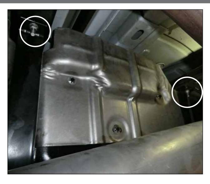
Step 9: It will be necessary to lower the fuel tank or remove the bed to gain access to the top of the fuel tank.
