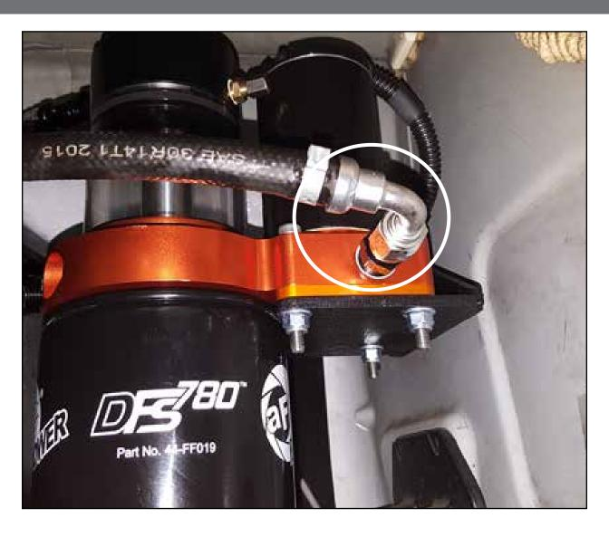
Step 18: Install the fuel inlet hose (silver  $90^{\circ}$  -6 AN fitting) onto the male -6 AN fitting on the fuel inlet port of the fuel manifold assembly and tighten.
