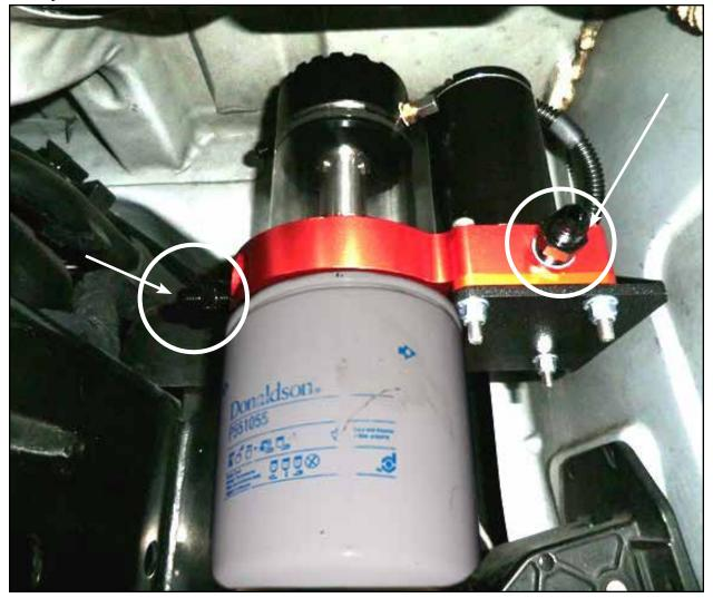
Step 8: Install the 2 x 3/8" NPT to -6 AN fittings into the fuel manifold assembly (as shown above).
