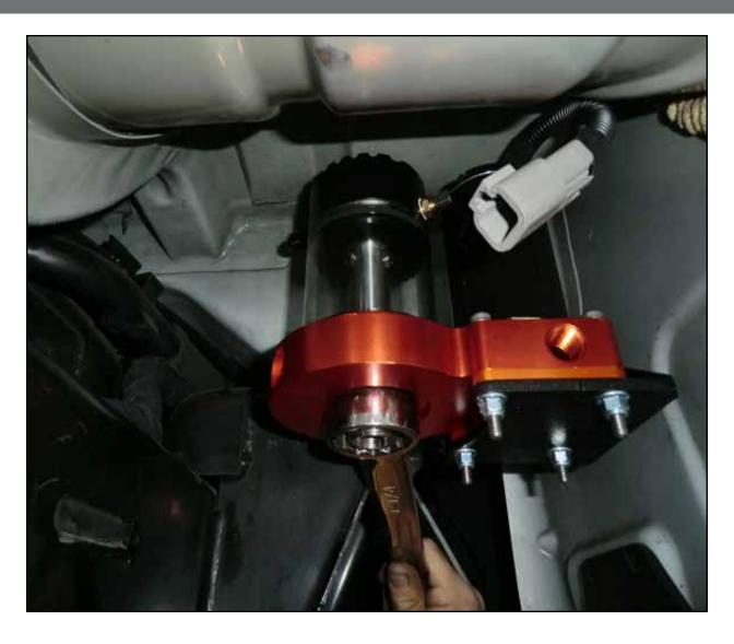
Step 5: Turn the sight glass to the desired angle and using a 1-1/4" wrench, tighten the center nut under the fuel manifold assembly.
