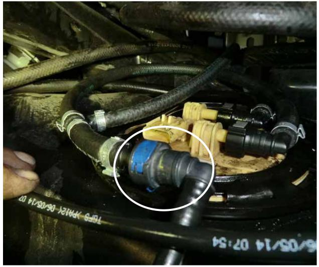
Step 17: Install the straight male quick disconnect fitting on the supplied fuel return hose into the female side of the stock fuel return line.
