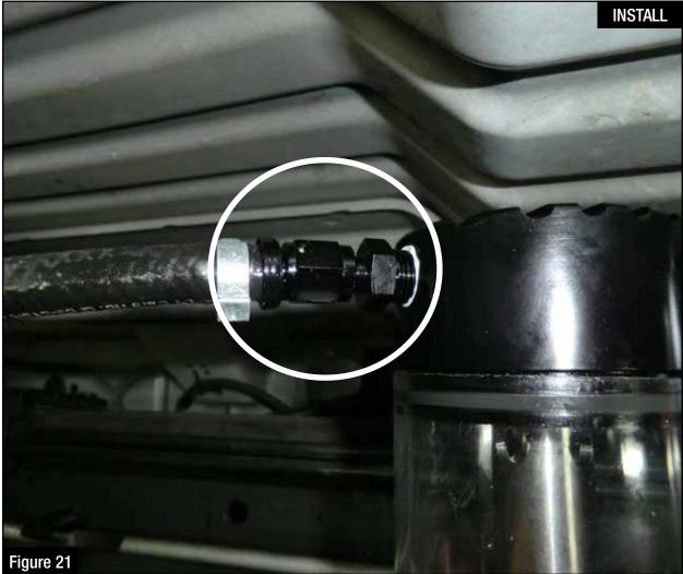
Step 22: Install the fuel return hose (-4 AN fitting) onto male -4 AN fitting on the top of the sight glass cover.
