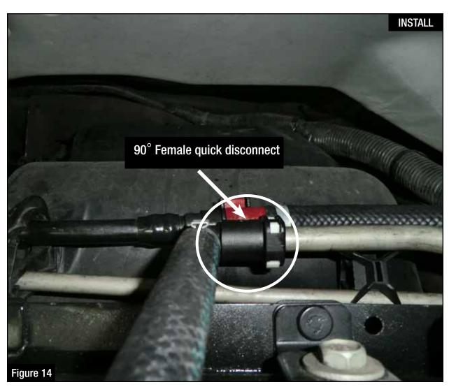
Step 15: Install the 90° female quick disconnect fitting on the supplied fuel outlet hose (black 90° -8 AN fitting - shown below) <u>onto the male side of the stock fuel</u> feed line.
