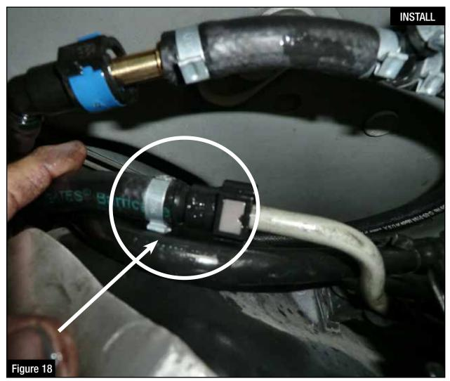
Step 19: Install the straight female quick disconnect fitting on the fuel return hose (shown be low) onto the male connection of the stock fuel return line.
