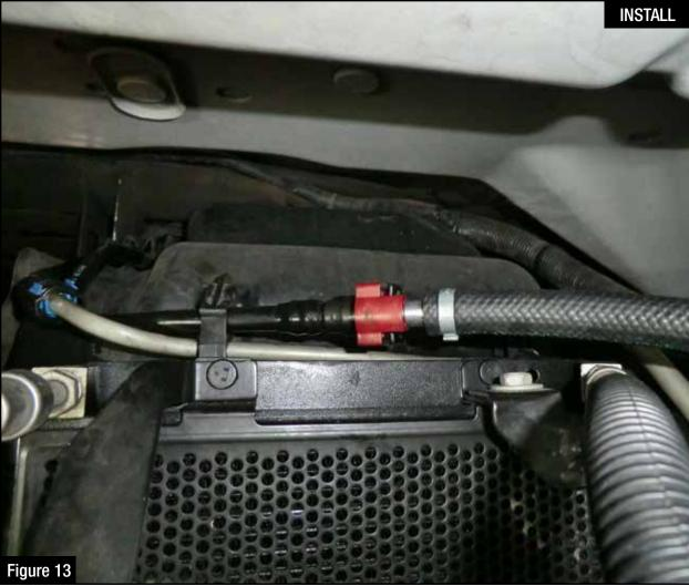
Step 14: Install the straight male quick disconnect fitting on the supplied fuel inlet hose (silver 90° -8 AN fitting - shown below) into the female side of the stock fuel feed line.
