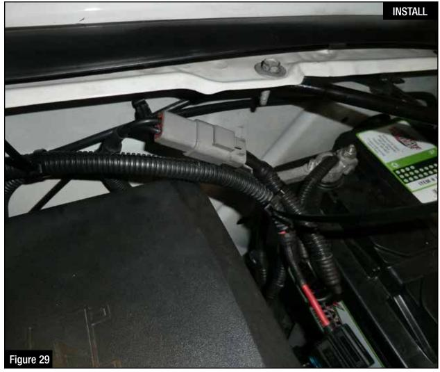
Step 32: Plug the supplied relay harness into the Deutsch connector on the power harness.
