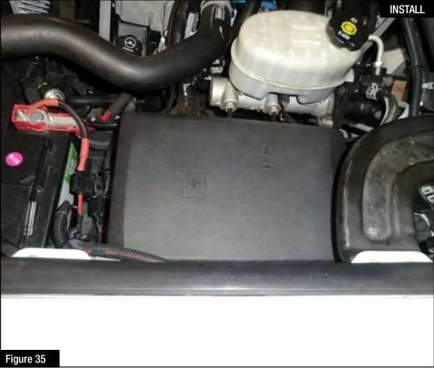
Step 39: Carefully route the power wire outside the fuse box and reinstall the cover (making Step 40: Organize the wire harnesses and secure with the remaining nylon cable ties. Step 41: Reinstall the corner brace using the hardware removed from Step 28.
