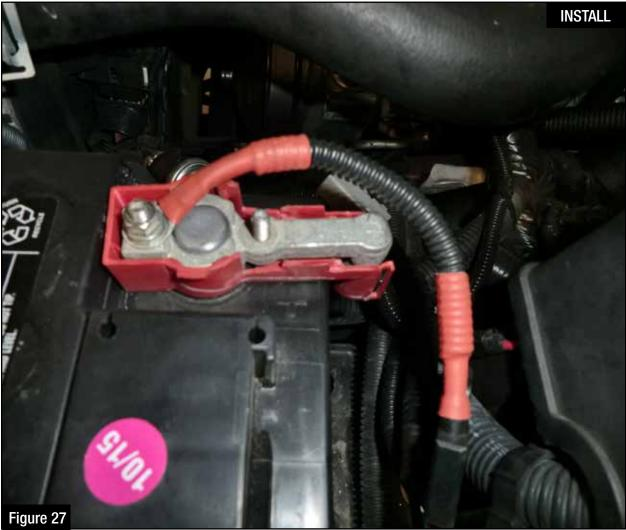
Step 30: Connect the red wire ring terminal to the positive side of the battery.
