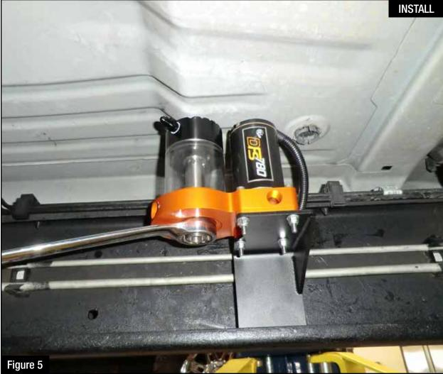
Step 8: Turn sight glass to the desired angle and using a 1-1/4" wrench, tighten the center nut under the fuel manifold.
