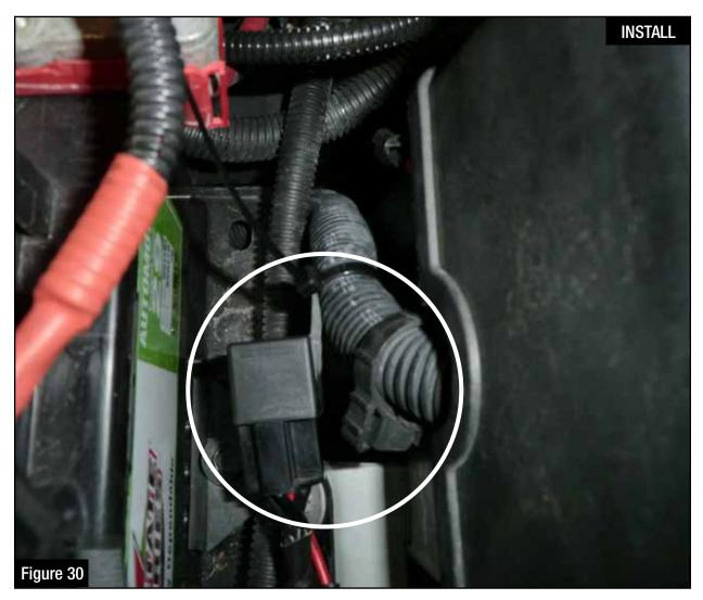
Step 33: Secure the relay harness using a supplied cable tie.
