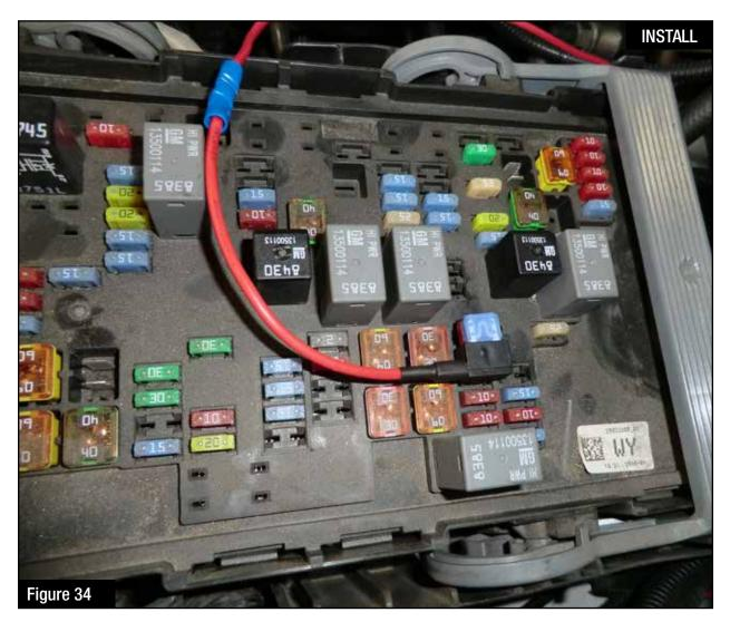
Step 38: Install the add a harness fuse adapter (with installed fuses) into the 12 volt source location chosen in Step 36.
