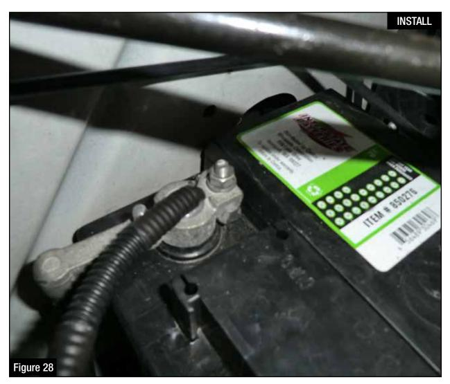
Step 31: Connect the black wire ring terminal on the power harness to the negative side of the battery.
