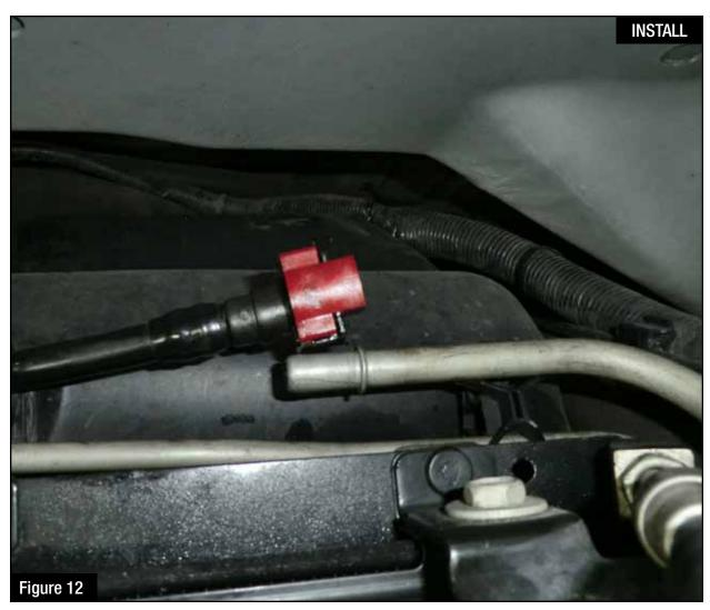
Step 13: Disconnect the 1/2" fuel feed line.
