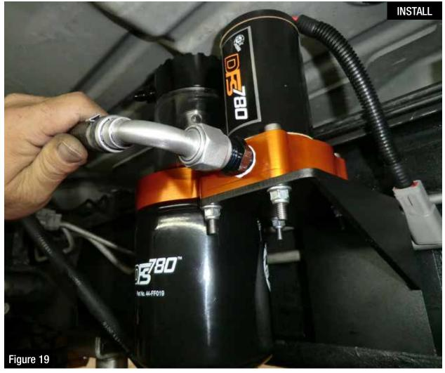
Step 20: Install the fuel inlet hose (silver 90° -8 AN fitting) onto the male -8 AN fitting on the fuel inlet port of the fuel manifold assembly.
