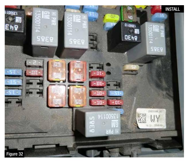
Step 35: Remove the fuse box cover. Step 36: Find a 12 volt source inside the fuse box that only comes on with the key in the "run" position.
