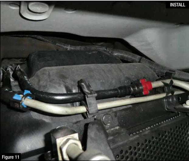
Step 12: Clean the area around the fuel lines to prevent dirt and debris from going into the lines.
