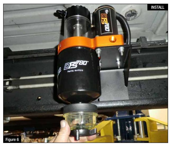
Step 9: Using a light oil, lube the gasket on the supplied fuel filter and install on the fuel manifold assembly. Thread the supplied water separator bowl onto the fuel filter.
