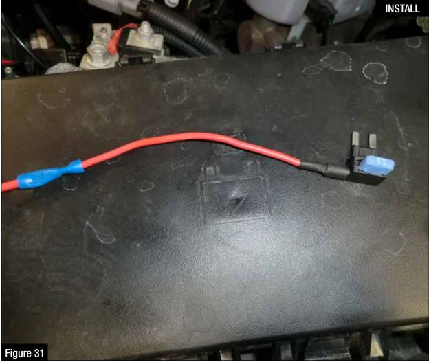
Step 34: Attach the power wire from the relay harness to the add a harness fuse adapter.
