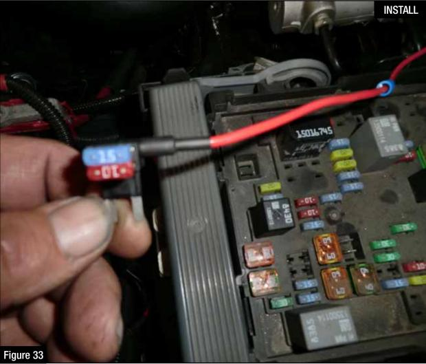
Step 37: Install the fuse removed in Step 36 into the open location on the add a harness fuse adapter (not in line with the wire).
