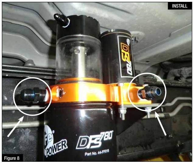
Step 11: Install the 2 x 3/8" NPT to -8 AN fittings into the fuel manifold assembly (as shown above).
