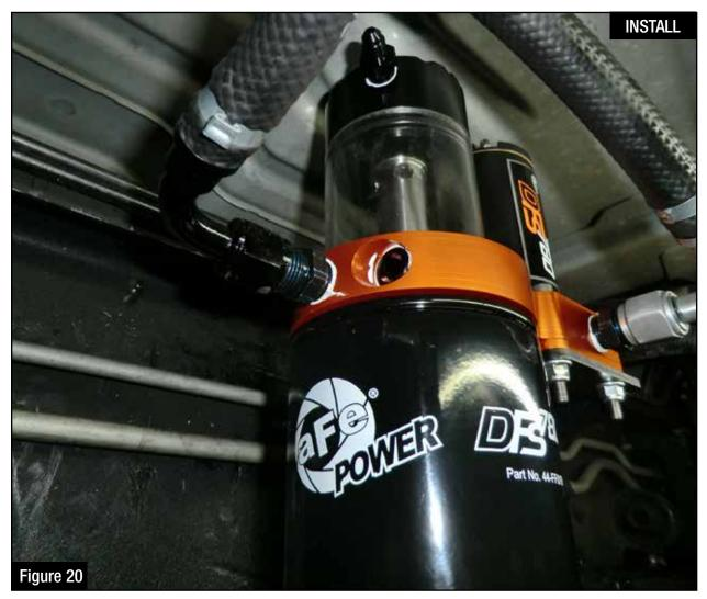
Step 21: Install the fuel outlet hose (black 90° -8 AN fitting) onto the male -8 AN fitting on the fuel outlet port of the fuel manifold assembly.
