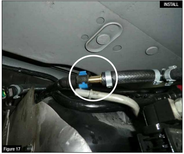
Step 18: Install the straight male quick disconnect fitting on the supplied fuel return hose ( shown below) into the <u>female side of the stock fuel ret</u>urn line.
