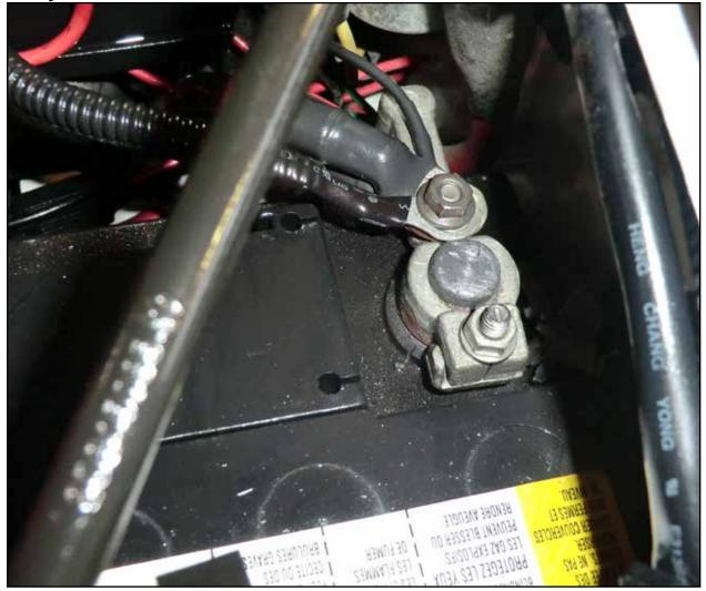
• Connect the black wire ring terminal on the power harness to the negative side of the battery.
