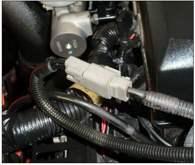
• Plug the supplied relay harness into the Deutsch connector on the power harness.
