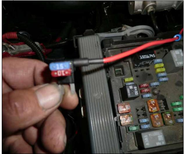
• Install the fuse removed on page 28 into the open location on the add a harness fuse adapter (not in line with the wire).
