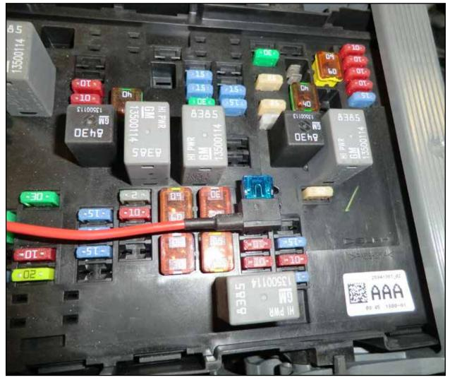
• Install the add a harness fuse adapter (with installed fuses) into the 12-volt source location chosen on page 28.
