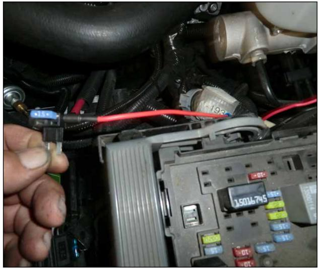
• Attach the power wire from the relay to the add a harness fuse adapter.
