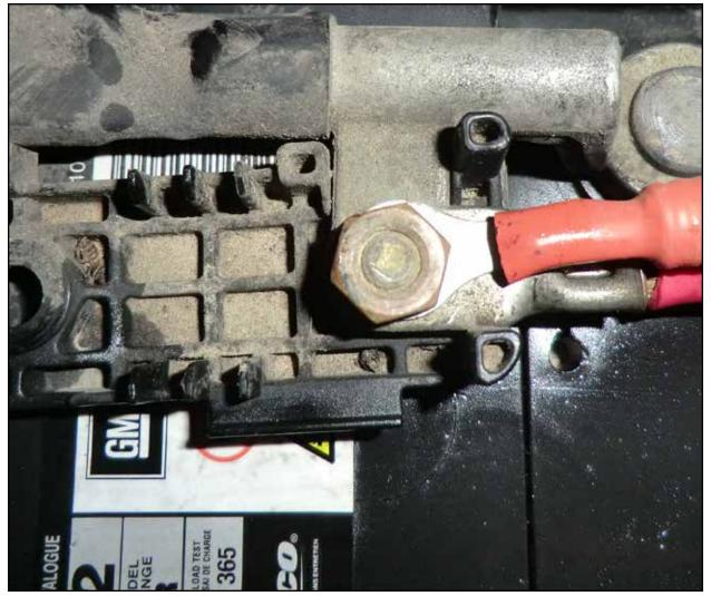
• Connect the red wire ring terminal on the power harness to the positive side of the battery.
