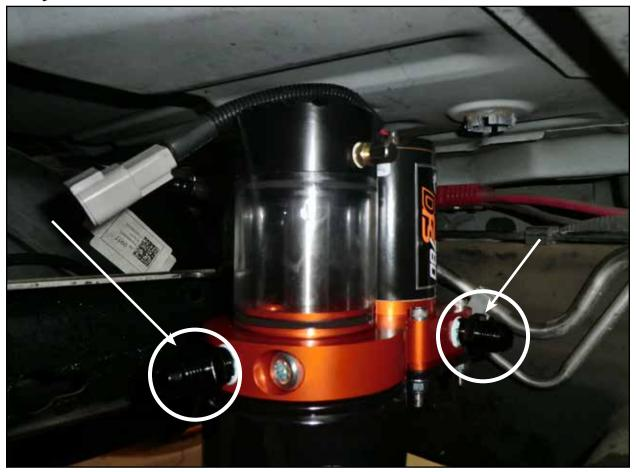
• Install the 2 x 3/8" NPT to -8 AN fittings into the fuel manifold assembly (as shown above).
