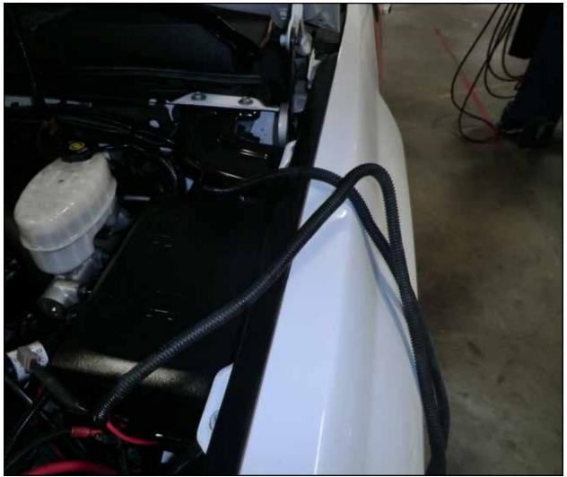
• Run the other end of the power harness along the frame into the engine compartment.
