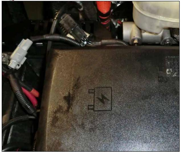
$\bullet$  Secure the relay harness using a supplied nylon cable tie.
