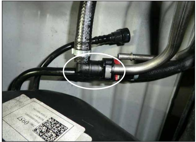
• Install the 90° female quick disconnect fitting on the supplied fuel outlet hose (black 90° -8 AN fitting - shown below) onto the male side of the stock fuel feed line.
