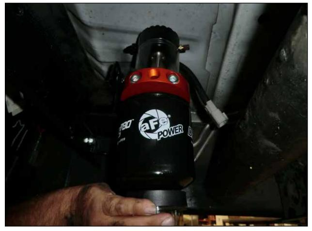
• Using a light oil, lube the gasket on the supplied fuel filter and install on the fuel manifold assembly. Thread the supplied water separator bowl onto the fuel filter.
