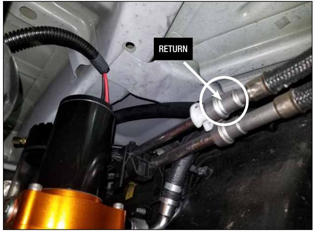
Step 17: Disconnect the factory fuel return line using a quick disconnect tool.
