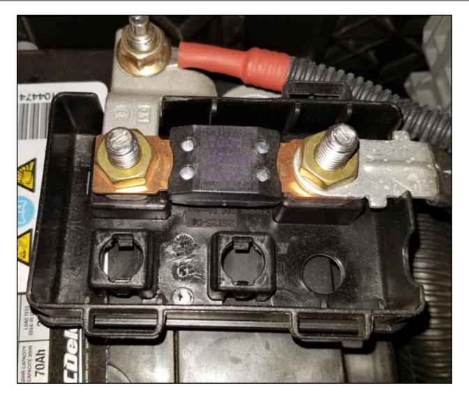
**Step 32:** Connect the red wire ring terminal on the power harness to the positive side of the battery.
