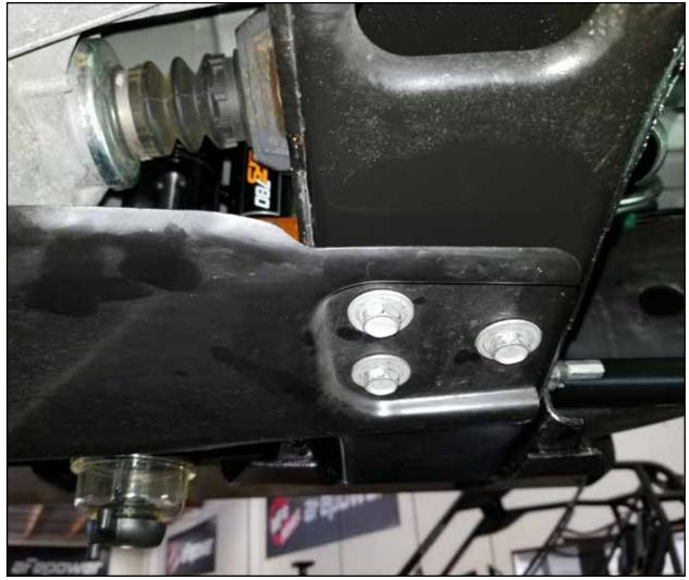
**Step 27:** Reinstall the factory transfer case skid plate using factory hardware.
