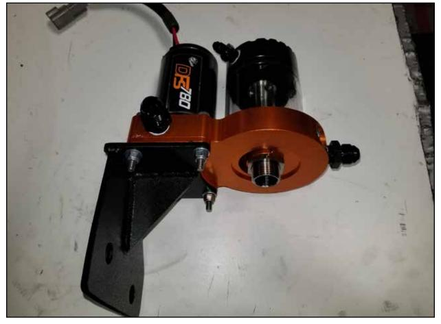
**Step 3:** Mount the supplied fuel manifold assembly to the carbon steel frame bracket using the supplied hardware and tighten.
