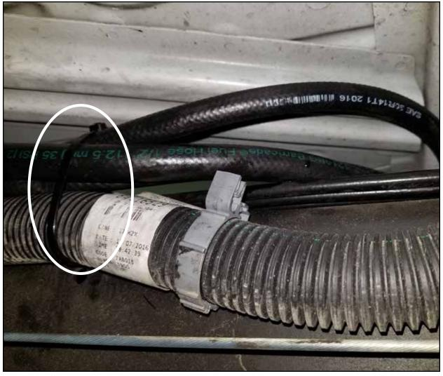
**Step 25:** Using the supplied nylon cable ties, secure the new hoses (as shown above).
