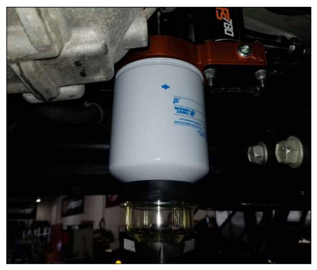
**Step 26:** Using a light oil, lube the gasket on the supplied fuel filter and install on the fuel manifold assembly. Thread the supplied water separator bowl into the fuel filter.
