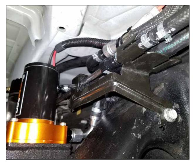
**Step 28:** From the inside of the frame, plug the Deutsch connector on the supplied power harness into the mating connector on the fuel pump motor.
