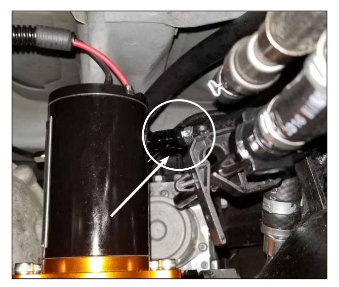
**Step 20:** Install the fuel return hose (-4 AN fitting) onto the male -4 AN fitting on the top of the sight glass cover and tighten.
