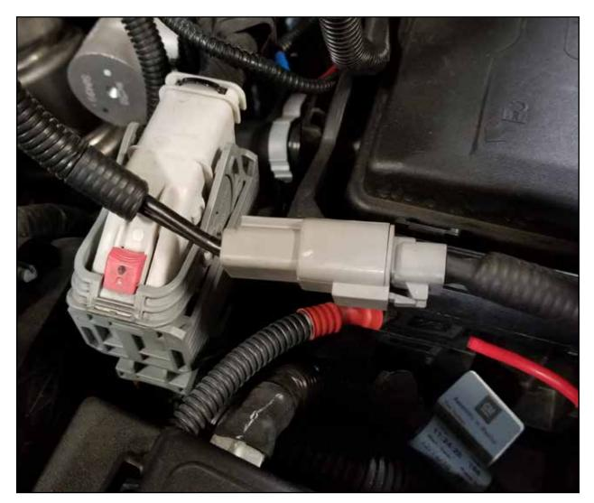
**Step 34:** Plug the supplied relay harness into the Deutsch connector on the power harness.
