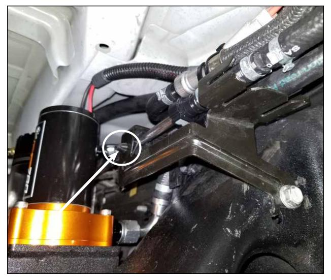
**Step 22:** Reinstall the factory fuel line retainer bracket.
