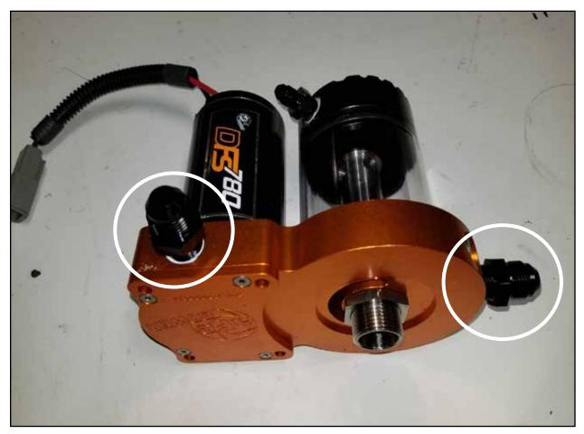
**Step 2:** Install the 2 x 3/8" NPT to -8AN fittings into the fuel manifold assembly (as shown above).
