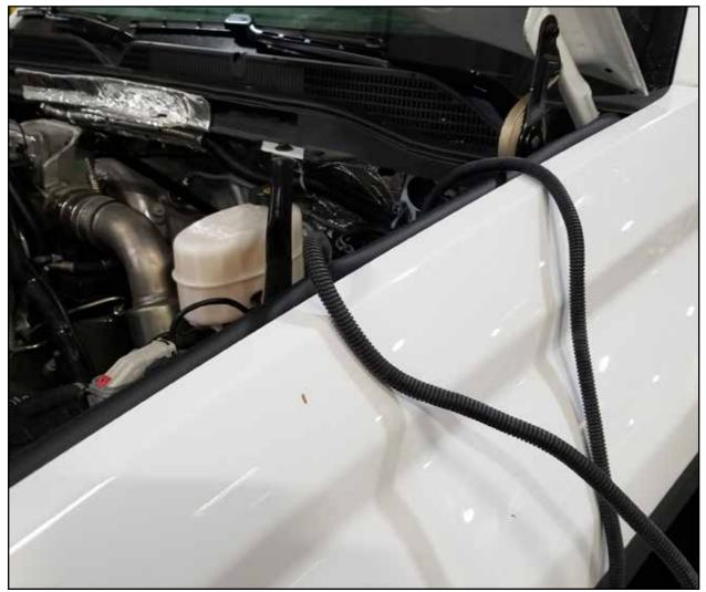
**Step 31:** Run the other end of the power harness along the inside of the frame into the engine compartment.
