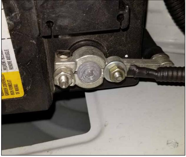
**Step 33:** Connect the black wire ring terminal on the power harness to the negative side of the battery.
