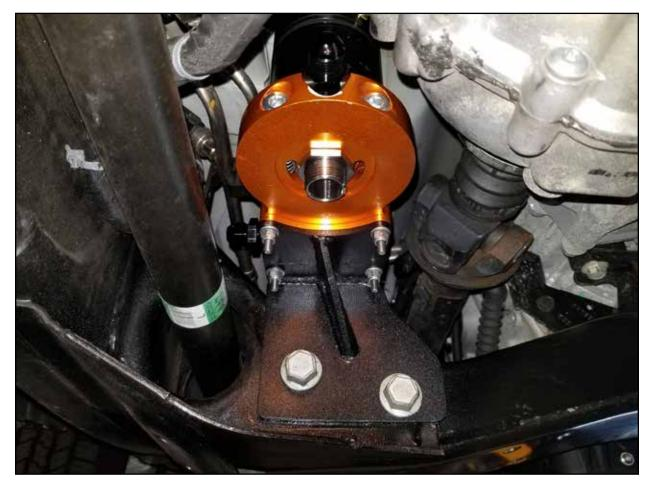
**Step 9:** Install the fuel manifold assembly and bracket (previously assembled) to the rear side of the transmission crossmember.
