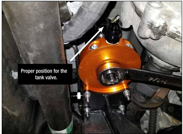
**Step 11:** Turn the sight glass to the desired angle and using a 1-1/4" wrench, tighten the center nut under the fuel manifold assembly.
