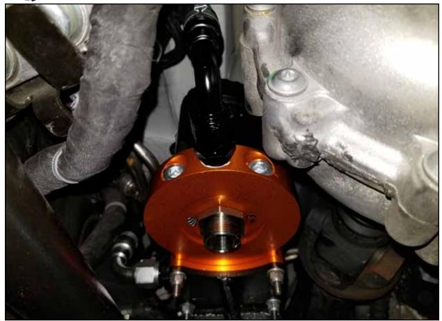
**Step 13:** Install the fuel outlet hose (black 90° -8 AN fitting) onto the male -8 AN fitting on the fuel outlet port of the fuel manifold assembly.
