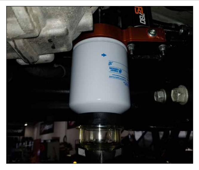
**Step 26:** Using a light oil, lube the gasket on the supplied fuel filter and install on the fuel manifold assembly. Thread the supplied water separator bowl onto the fuel filter.
