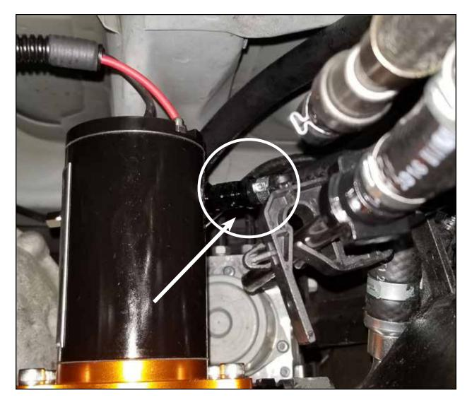
**Step 20:** Install the fuel return hose (-4 AN fitting) onto male -4 AN fitting on the top of the sight glass cover.
