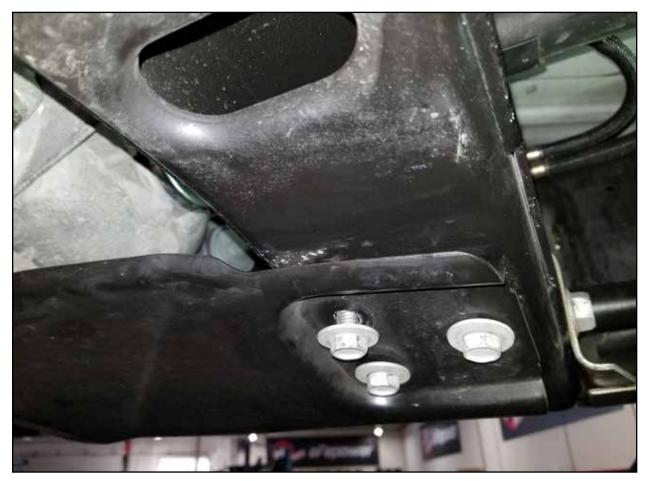
**Step 6:** Remove the factory transfer case skid plate (if applicable). Save hardware and skid plate for reinstallation.
