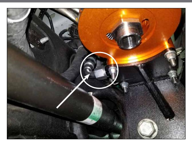
**Step 12:** Install the fuel inlet hose (silver 90° -8 AN fitting) onto the male -8 AN fitting on the fuel inlet port of the fuel manifold assembly.
