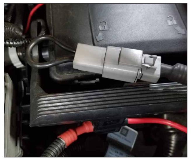
**Step 36:** Make sure that all fittings are tight. Install the priming jumper onto the Deutsch connector on the power harness. The fuel pump motor will turn on. Watch to see if the sight glass fills with fuel. If the sight glass does not fill with fuel, use the tank valve (on the top of the sight glass cover) to release any trapped air. If the sight glass still does not fill, try starting the engine. Check for any leaks.
