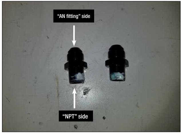
**Step 1:** Apply Teflon tape with PTFE or Teflon paste with PTFE to the 2 x 3/8" NPT to -8 AN fittings.
