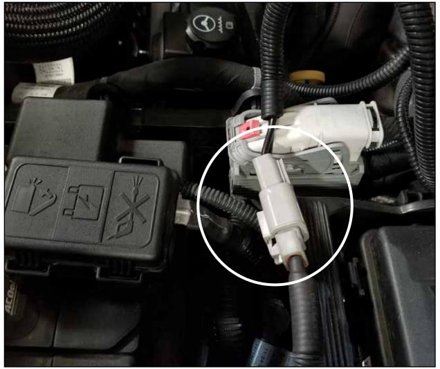
**Step 38:** Plug the pressure switch harness onto the Deutsch connector on the power harness. **Step 39:** Organize any of the loose wire harnesses and secure with the remaining nylon cable ties.
