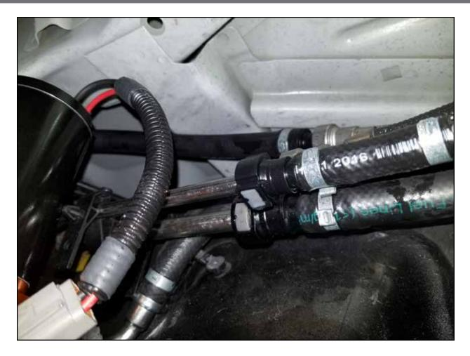
**Step 18:** Install the straight female quick disconnect fitting on the fuel return hose (shown below) onto the male connection of the stock fuel return line.
