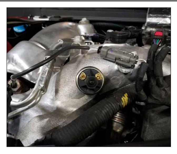
Step 34: Install the supplied pressure switch into the intake manifold (1/8" NPT).
