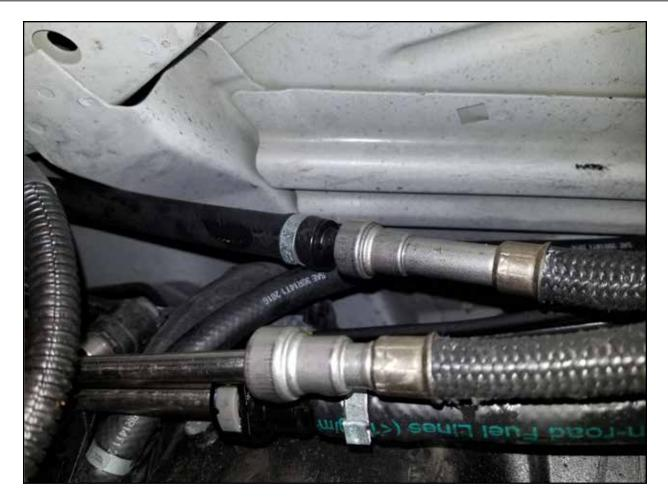
Step 16: Install the male quick disconnect fitting on the supplied fuel outlet hose (black  $90^{\circ}$  -8 AN fitting shown below) into the female side of the stock fuel feed line.
