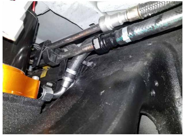
**Step 15:** Install the straight female quick disconnect fitting on the supplied fuel inlet hose (silver 90° -8 AN fitting shown below) onto the male side of the stock fuel feed line.
