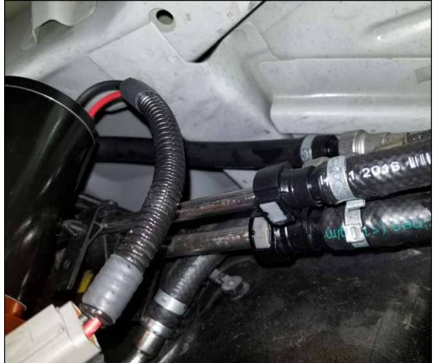
**Step 19:** Install the straight male quick disconnect fitting on the supplied fuel return hose (shown below) into the female side of the stock fuel return line.
