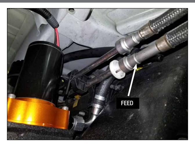
**Step 14:** Disconnect the factory fuel feed line using a quick disconnect tool.
