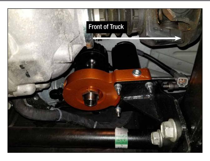
**Step 9:** Install the DFS pump and bracket (previously assembled) to the rear side of the transmission cross member.
