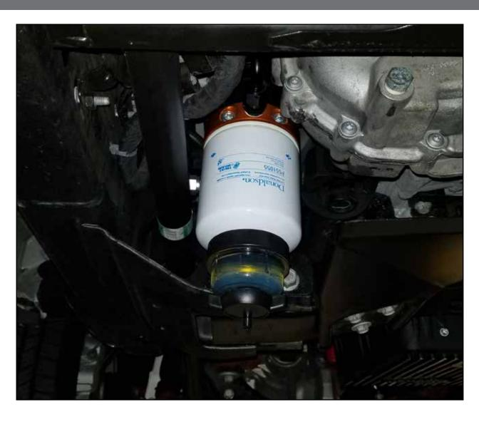
Step 40: Start the truck and let idle while checking for any leaks.
