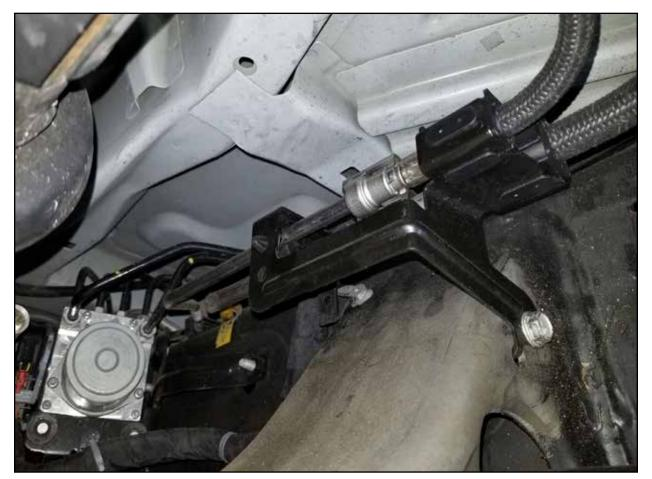
Step 4: Locate the fuel lines on the driver side near the transfer case (shown in picture).
