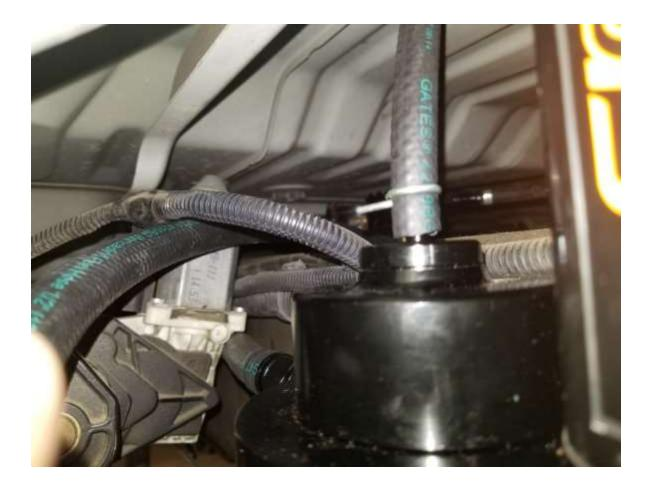
**35.** Carefully route the ¼" hose to the fitting on the top of the fuel manifold assembly, making sure not to kink the hose or allow it near moving parts. Carefully mark and then cut the hose to the correct length. Using a spring clamp, attach the hose to the nipple on the top of the air chamber on the fuel manifold assembly.
