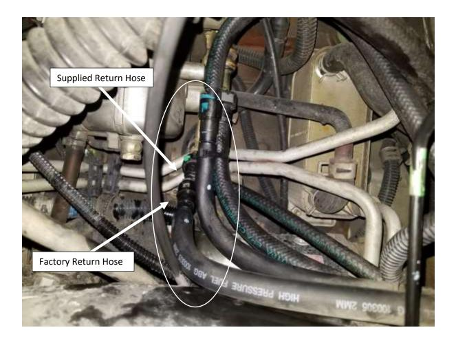
**34.** Disconnect the factory fuel return line. Attach the supplied fuel return hose between the male and female factory fuel fittings. Push all connections togethers.
