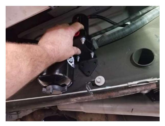
**23.** Place the fuel manifold assembly on to the truck and mark the three holes using the carbon steel frame bracket.
