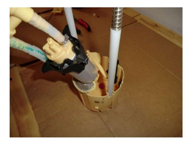
**10.** Remove the factory fuel pump, suction line and return line from the fuel sender assembly.
