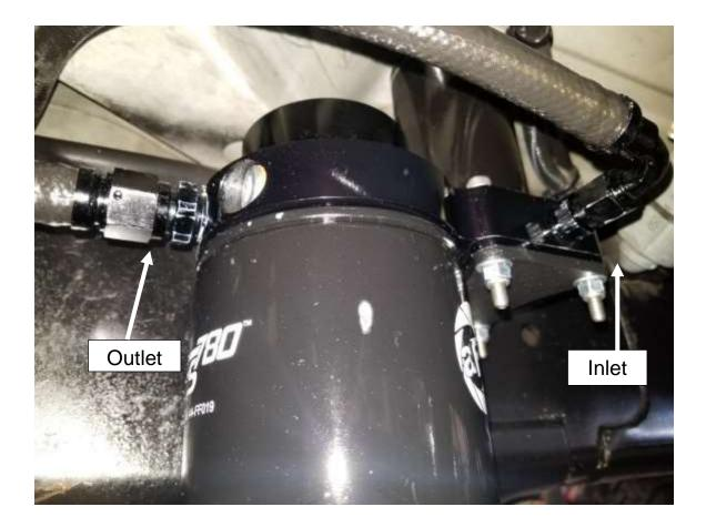
**33.** Attach the fittings to the inlet & outlet ports of the fuel manifold assembly. Make sure all connections are tight.
