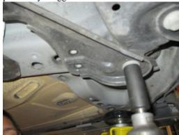
8. Reinstall the rear main subframe brace.
