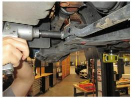
8. Loosen and remove the two bolts that secure the exhaust hanger to the subframe.
