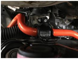
4. You can now raise the subframe back up into position. Be careful to make sure nothing is binding or pinching. You can use a pry bar to help align the subframe bolts. **Do not fully tighten bolts yet, just snug to hold position.**
