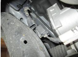
12. Using a screw jack, support the subframe, then remove the left and right side forward sub frame bolts. We chose to place the screw jack forward on the subframe near the lower control arms, this is helpful in the next step.
