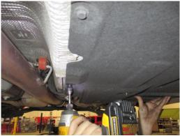
6. Remove the rear main subframe brace by removing the four nuts and bolts that secure it to the vehicle.
