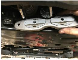
9. Loosen and remove the left and right side subframe brackets by loosening and removing the bolts that secure them in place.
