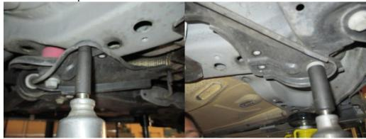
10. Loosen and remove the bolts that secure the transaxle to the sub frame. OEM mount may differ from photo, aftermarket mount shown on vehicle.
