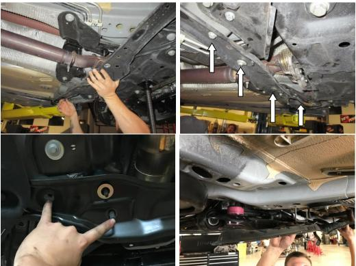
7. Loosen and remove the bolts that secure the forward sub frame brace
