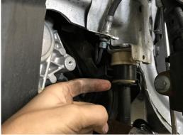
13. Slowly lower the subframe, be careful to ensure that you are not binding on anything and that all electrical connections and lines are free and not under tension. We were able to achieve this step by rotating the subframe back, and not completely dropping it from the vehicle. In this step be careful not to pull too far, as the steering rack is still connected to the steering shaft.
