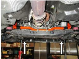
14. Alternate method to step 13. Remove the 3 bolts that secure the steering rack to the subframe. Using a ratchet strap secure the tie rods to the strut assemblies. This will keep them in place during the next step as the sub frame is lowered. Failure to do this could cause damage to the steering.
