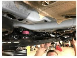
9. Re-attach the rear exhaust hanger bracket to the subframe.
