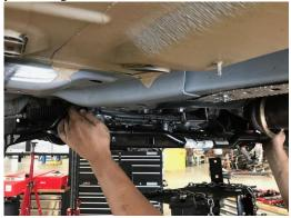
17. Before removing the brackets, take time to note the orientation of the OEM brackets, the holes are offset and this orientation will need to be followed upon reinstallation.
