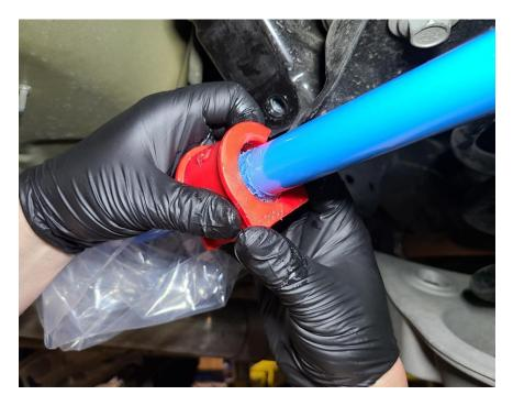
Install the provided billet brackets onto the bushings and reuse the factory bolts. Make sure the grease fittings are pointing outward towards the wheels. Shift brackets up before full tightening the bracket bolts.
