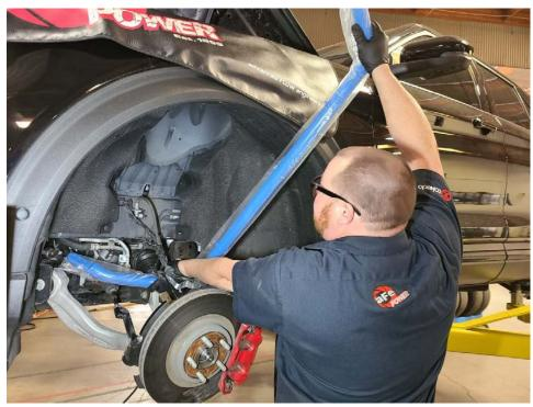
10F It is extremely difficult to spread open the front bushings to install on the bar. Instead, it is easier to just insert it from the end and slide it into place.
