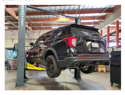
2R Note: Our test vehicle has an aFe exhaust installed, so if you have the stock exhaust (Below), you will need to drop it slightly to access the heat shield hardware.
