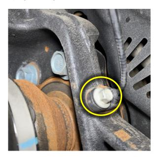
Next, loosen the lower strut <u>nuts</u> using a 24mm Socket. Note: The bolt itself is knurled and pressed into the strut/upright holes, Do NOT try to spin these.
