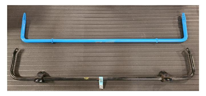
Install the aFe CONTROL sway bar in the same manner as factory removal. Tip: It's a good idea to keep the sway bar in the poly bag it ships in when inserting it into the car. This will avoid any unnecessary scratches to the bar. Once the bar is in place, remove the poly bag.
