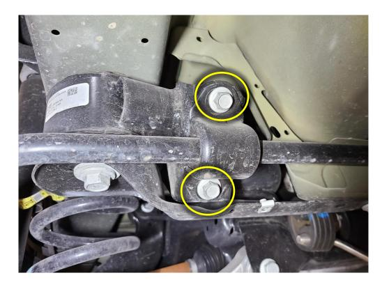
5R Remove the bar towards either side of the vehicle. (Wheels are removed for clarity purposes)
