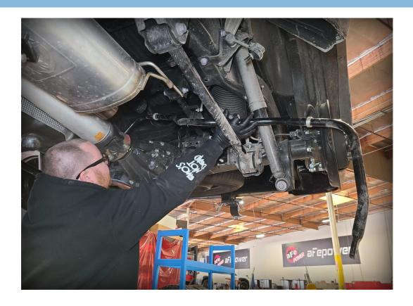
5R Reinstall the aFe CONTROL sway bar in the same manner as removal. Tip: Keep the poly bag on the sway bar during installation. This will help prevent scratches when fishing the bar in.
