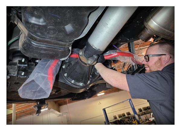
Lube the inside surface of the bushings with the supplied silicon grease. Install the bushings onto the bar. Bushing should be outboard of the centering rings.
