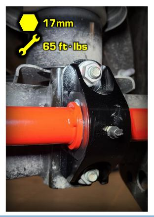
Attach the end link to the bar using the factory nuts and fully tighten. The hole furthest from the end is the stiffest setting. (Shown) The hole closest to the end is the softest setting. Tip: Add some thread locking compound to the end link stud to ensure long lasting tightness.
