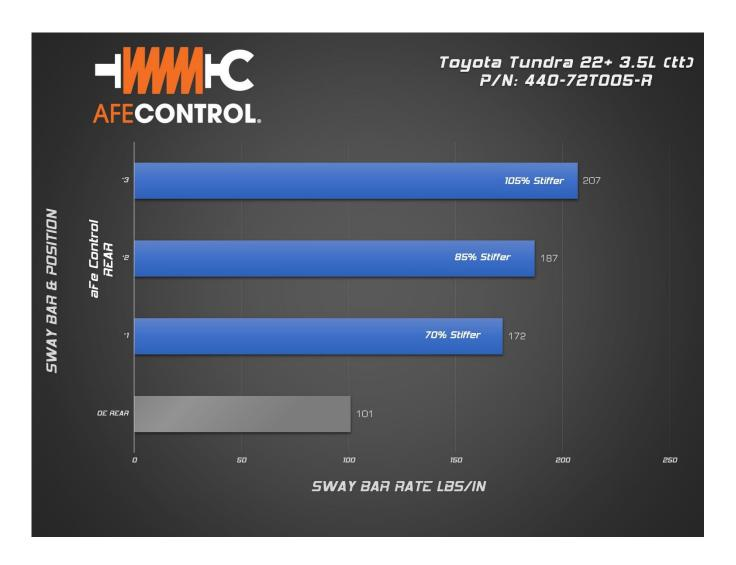
Suggested Settings for Towing, Payload, or Bed Rack with storage: Position #3 Hard Stiffness (Hole furthest from the end)
