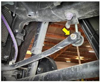
4R Unbolt the sway bar bushing mount nuts (4) and remove the sway bar from the vehicle. Retain this hardware for reinstallation.
