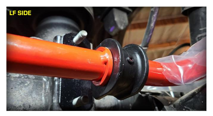
6R Install the included bridge plate onto the bushing bracket studs on the rear end differential. The small metal strip in the center of the plate should face the rear axle. Install the aFe billet bushing brackets onto the bushings and fasten them to the axle using the OE nuts.
