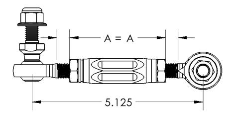
Tighten jam nuts with the rod ends clocked 90° apart. Left side shown below.
