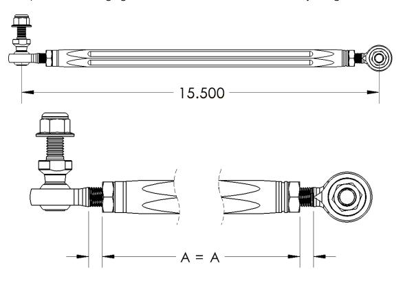
For cosmetic purposes, to avoid scratching the blue anodizing, we suggest using an aluminum adjustable wrench or applying masking tape to a normal wrench. The sleeve size is 3/4" and the jam nuts are 11/16".
