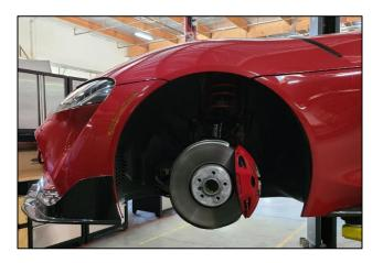
3F Unfasten the left end link from the strut using a T30 socket to hold the stud and a 16mm wrench to undo the nut.
