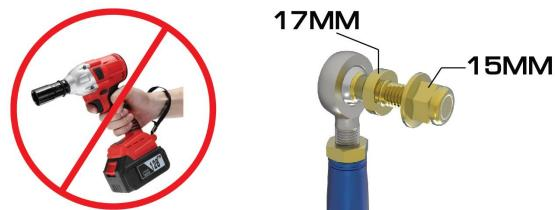
7F You should now have the end links installed with only the right-hand jam nut loose to clock the rod end angle.
