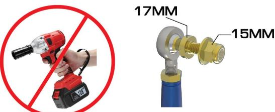
7R Repeat for the passenger side. Clocking and positioning will be a mirror image of the left. Reinstall wheels and torque lug bolts to 103 ft lbs.
