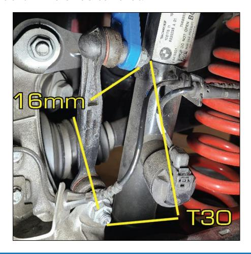
4R Set the aFe Control end link to 5.125" center to center. Make sure to have equal thread engagement for each rod end when adjusting.
