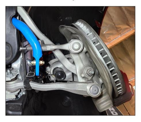
8F Repeat for the passenger side. Clocking and positioning will be a mirror image of the left. Reinstall wheels and torque lug bolts to 105 ft lbs.
