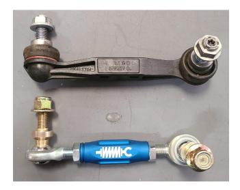
Optional: For cosmetic purposes, to avoid scratching the blue anodizing on the sleeve, we suggest using an aluminum adjustable wrench or applying masking tape to a normal wrench. The sleeve size is 3/4" and the jam nuts are 11/16".
