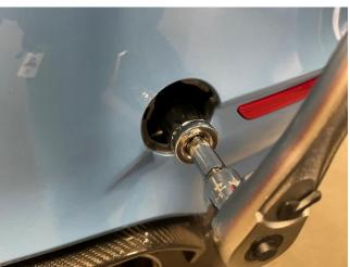
4. Attach the hook to the stem using the included M12 bolt with a 15mm socket and firmly tighten it.
