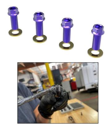
(Optional) Apply anti-seize onto the first half of the bolt threads.
