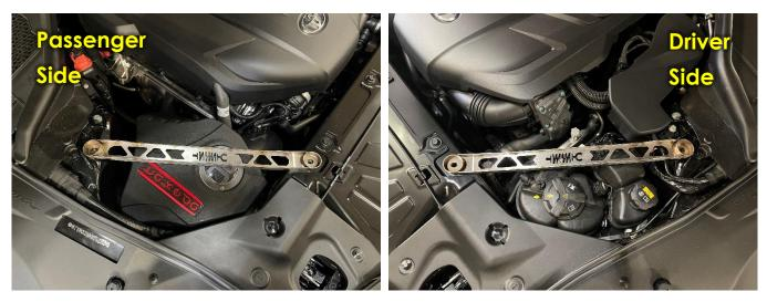
4. Install all (4) M10 bolts with washers by hand first. Then torque down the bolts to 30 ft·lbs with a 12mm socket and you're done.
