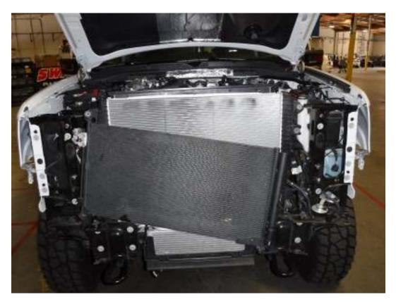
45. Remove the two (2) bolts securing the power steering cooler to the vehicle using a 10mm socket.
