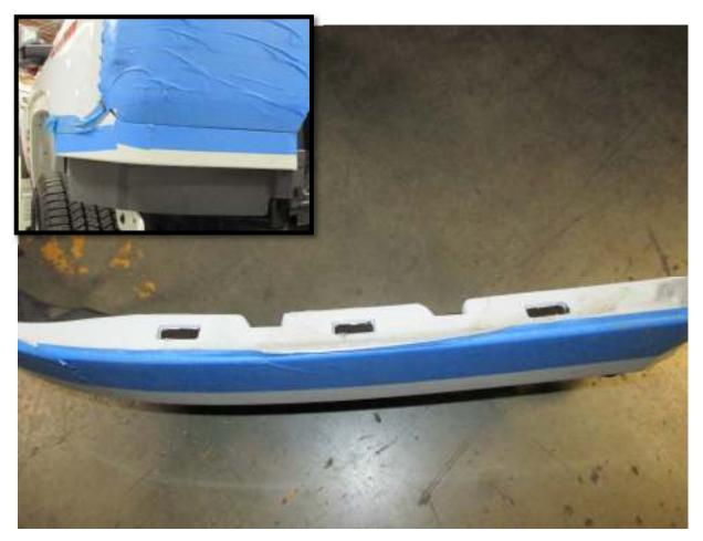
16. Unclip the air deflectors from underneath the headlights and remove them from the vehicle.
