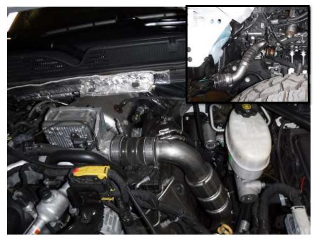
20. Loosen the clamps for the hot side intercooler tube at the turbo outlet and intercooler inlet on the driver side of the vehicle using a 11mm socket.21. Remove the hot side intercooler tube from the bottom of the vehicle.
