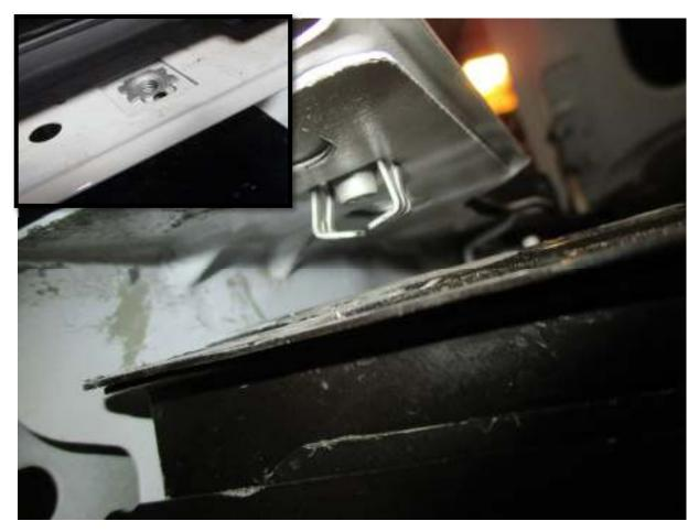
40. Remove both headlight mounting clips from the fenders, by squeezing the ends underneath the fender together and pulling it out of the top.
