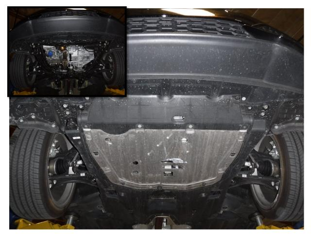
10. Remove all the bolts and clips securing the belly pan to the vehicle.
