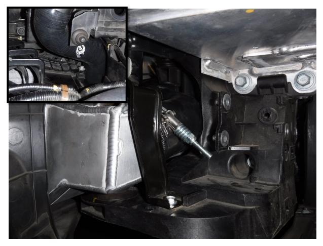
52. Install the supplied silicone hose along with one (1) of the supplied 2-3/8" clamps onto the intercooler from the top (do not tighten the clamp yet).
