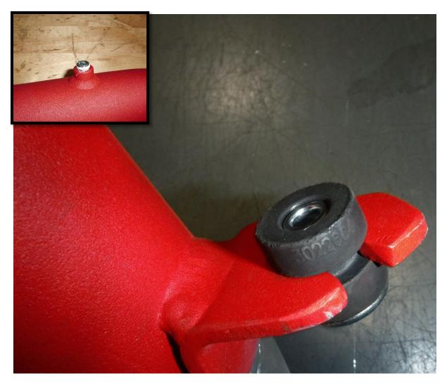
41. Transfer the rubber mounting grommet onto the supplied aFe hot side intercooler tube.
