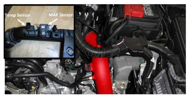
54. Remove the temp sensor and MAP sensor from the factory intercooler tube.
