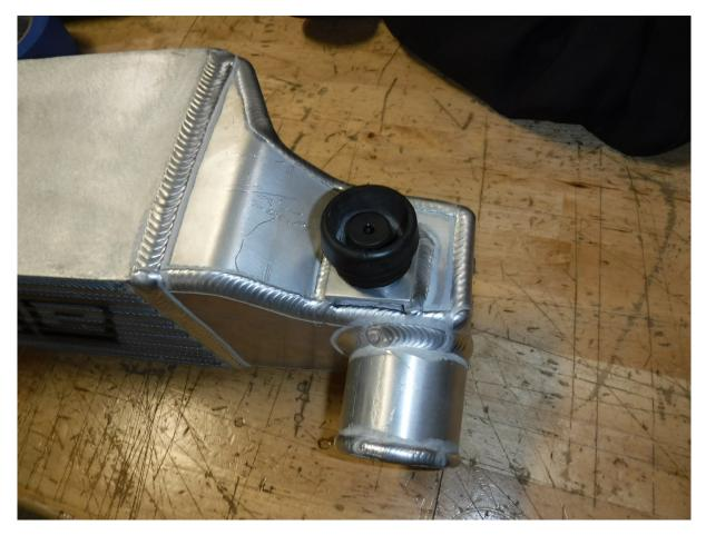
35. Transfer all four (4) of the mounting grommets onto the supplied aFe intercooler.
