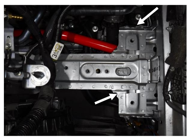
12. Remove the two (2) screws that secure the hot side intercooler tube plastic adapter to the vehicle.
