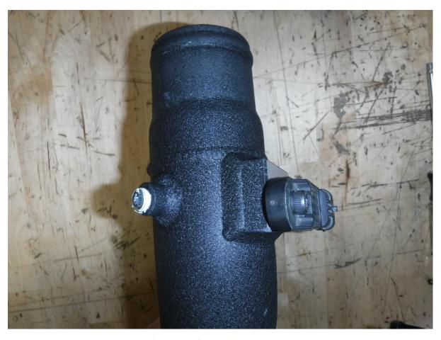
33. Remove the MAP sensor from the factory upper cold side intercooler tube.
