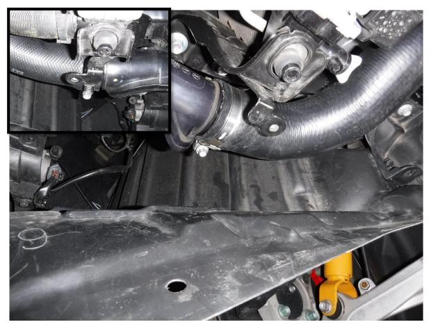
17. Loosen the clamps securing both intercooler tubes to the intercooler.
