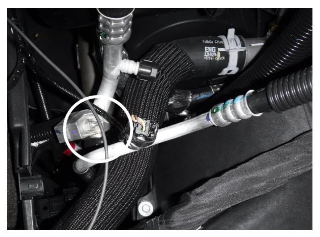
9. Locate the hot side intercooler tube on the passenger side of the vehicle, below the air conditioning line, then loosen the clamp securing the tube to the turbo outlet tube.
