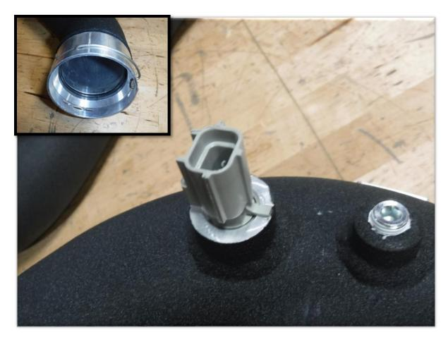
42. Remove the temperature sensor from the factory cold side intercooler tube by gently lifting the tab and twisting it counter clockwise 1/4 turn, then pulling it out of the tube.
