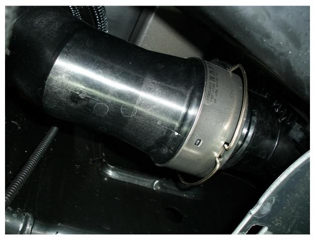
15. Underneath the vehicle on the driver side, disconnect the quick connect adapter connecting the cold side intercooler tube to the intercooler.
