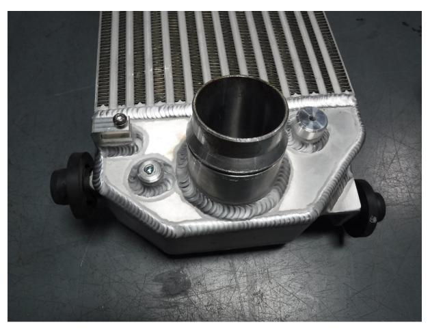
Note: Be sure to use thread sealant on the plugs or sensors to prevent any leaking
