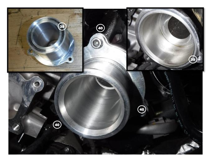
Note: Be sure to lubricate the O-ring with grease prior to installation.
