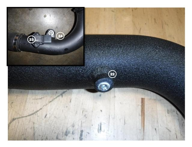
Note: Be sure to use thread sealant on the plug or sensor to prevent any <u>leaking</u>
