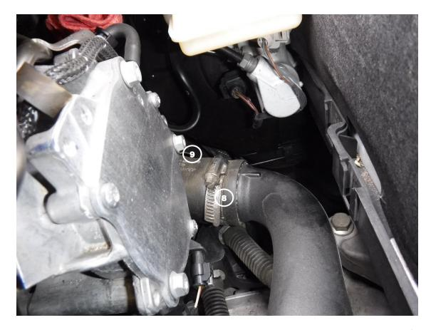
10. Loosen the two (2) clamps securing the hot side intercooler tube onto the turbo outlet (8.)
