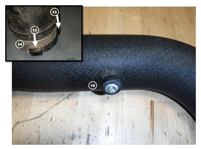
Note: The retaining clips will need to be removed from both factory charge pipes for reuse with the aFe charge pipes
