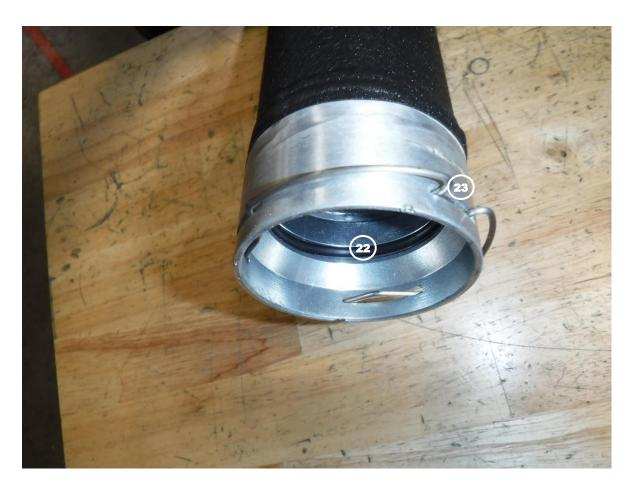
Note: Be sure to lubricate the O-ring with grease to prevent it from tearing during installation.
