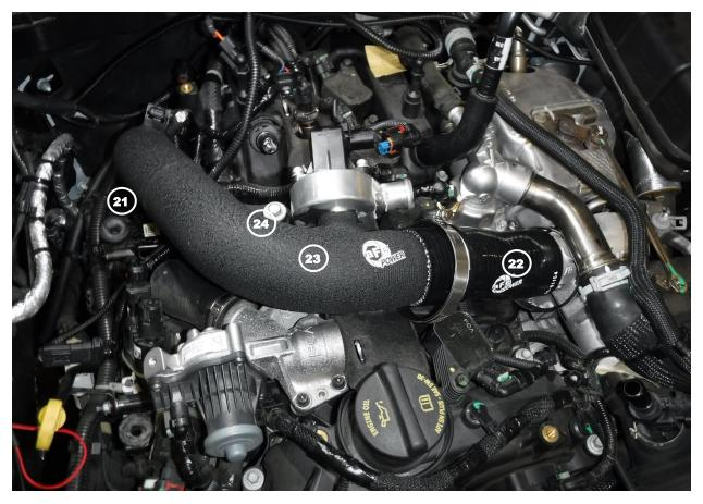
Note: Be sure to thoroughly clean all oil residue off of the connections before installing any of the aFe couplings onto the vehicle.
