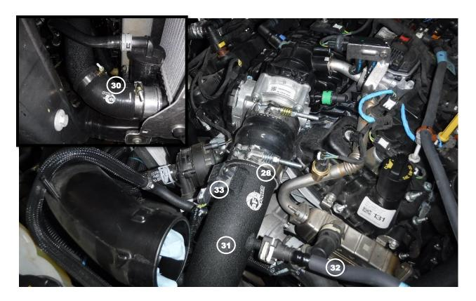
Note: Be sure to thoroughly clean all oil residue off of the connections before installing any of the aFe couplings onto the vehicle.
