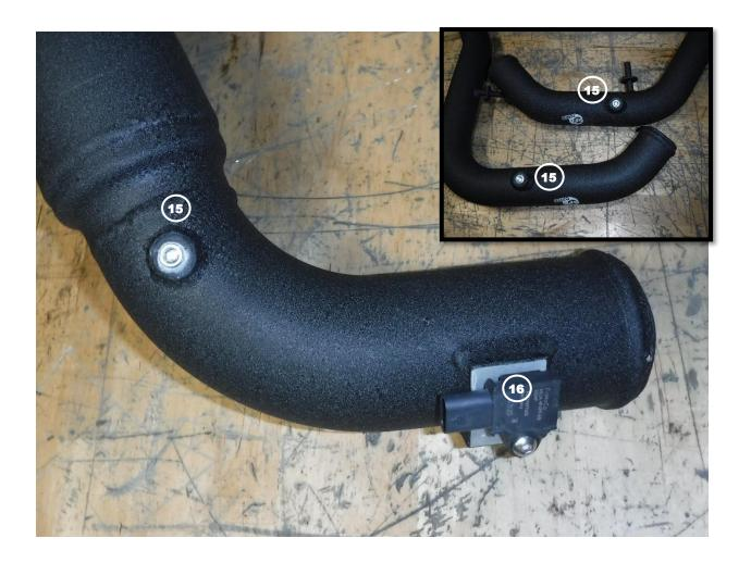
Note: Be sure to use thread sealant on the plugs or sensors to prevent any leaking.
