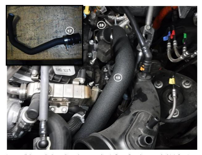
24. Install the supplied aFe silicone hump coupling 2.5"ID x 4"L and one supplied 2.85" springloaded T-Bolt clamp onto the aFe hot upper driver side charge pipe (17) then tighten the clamp.
