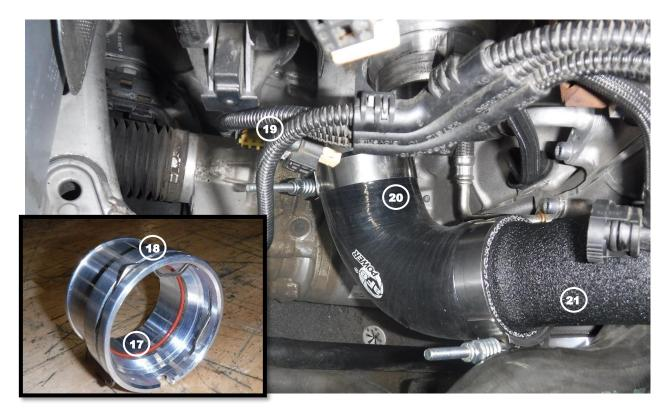
Note: Be sure to lubricate the O-ring with grease to prevent it from tearing during installation.
