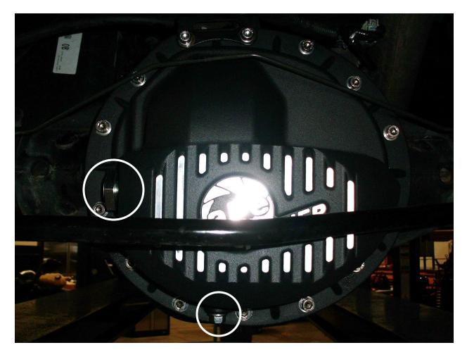
14. Install the supplied M12x1.25 drain plug and crush washer into the bottom of the cover.
