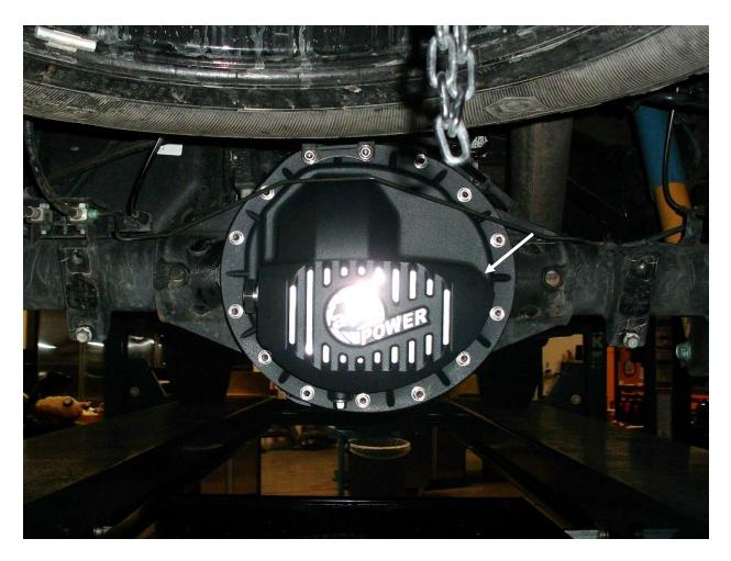
16. Using the top fill port, fill the aFe differential cover with new gear oil. Fill until gear oil runs out of the 1/8" NPT port on the side of the cover (about 3 ½ quarts).
