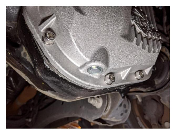
18. Install the supplied M12x1.25 drain plug and crush washer into the bottom of the cover.
