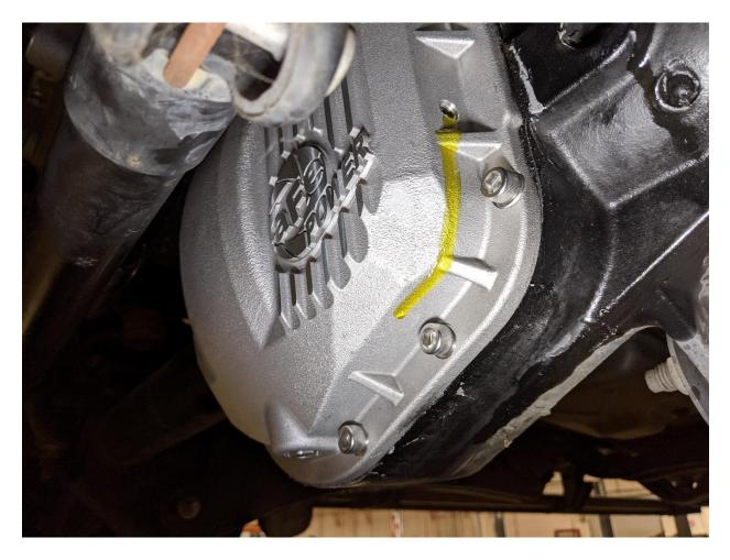
20. Using the top fill port, fill the aFe differential cover using new gear oil. Fill until gear oil runs out of the 1/8" NPT port on the side of the cover (about 4 quarts).
