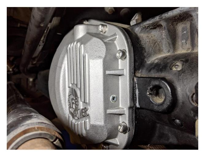
22. Install one (1) 1/8" NPT plug into the side of the cover.
