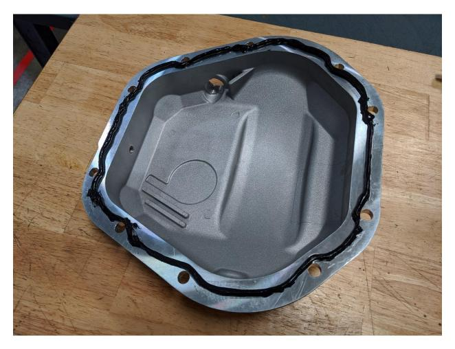
13. Hold the supplied aFe differential cover up to the gasket surface to make sure you will be able to maneuver it into place easily.
