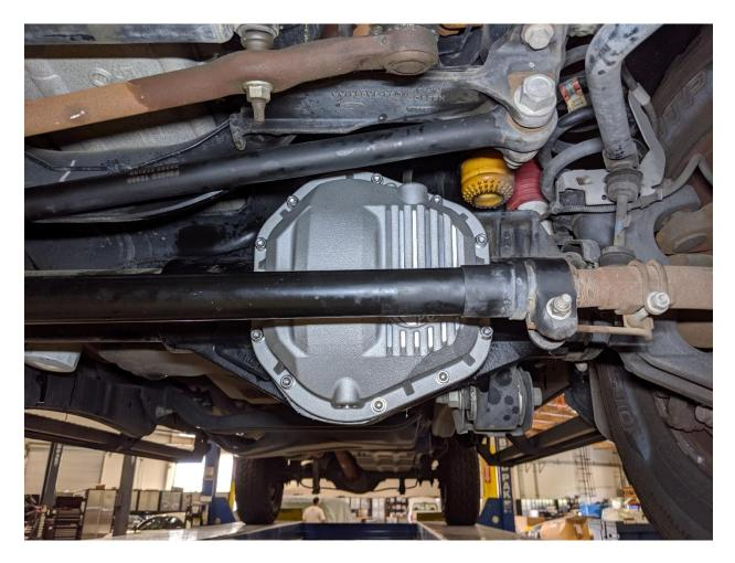
15. Hold the aFe differential cover into position, aligning the screw holes. Install four (4) of the supplied 3/8"-16x1" socket head screws and flat washers into separate sides of the cover to hold it in place.
