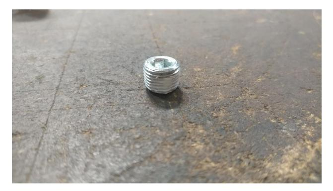
21. Apply Teflon pipe sealant to the threads of the two (2) supplied 1/8" NPT plugs.
