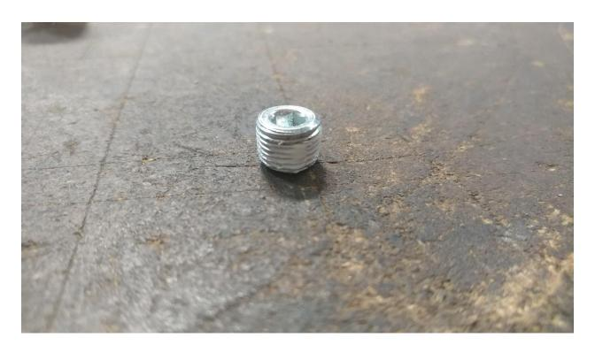
22. Apply Teflon pipe sealant to the threads of the supplied  $1/8^{\prime\prime}$  NPT plug.
