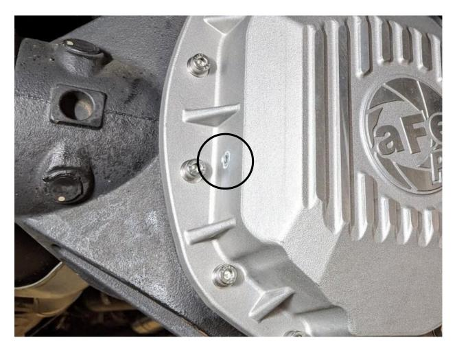
24. Install the 1/8" NPT plug into the side of the cover.
