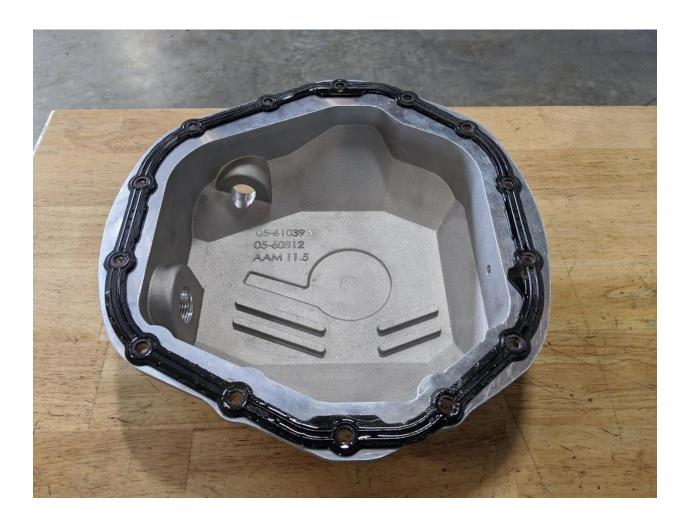
14. Line up the gasket removed in Step 10 to the supplied aFe differential cover.
