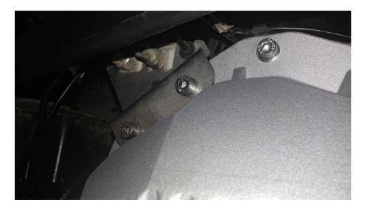
16. If applicable, reinstall the brake line bracket using two (2) supplied M8x1.25x40 socket head screws, two (2) spacers, and four (4) flat washers.
