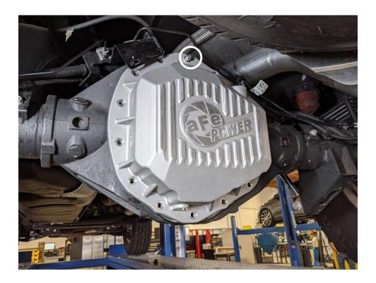
15. Hold the aFe differential cover and gasket in position, aligning the screw holes. Install one (1) of the supplied M8x1.25x30 socket head screws and flat washers into the top of the cover to hold it in place.
