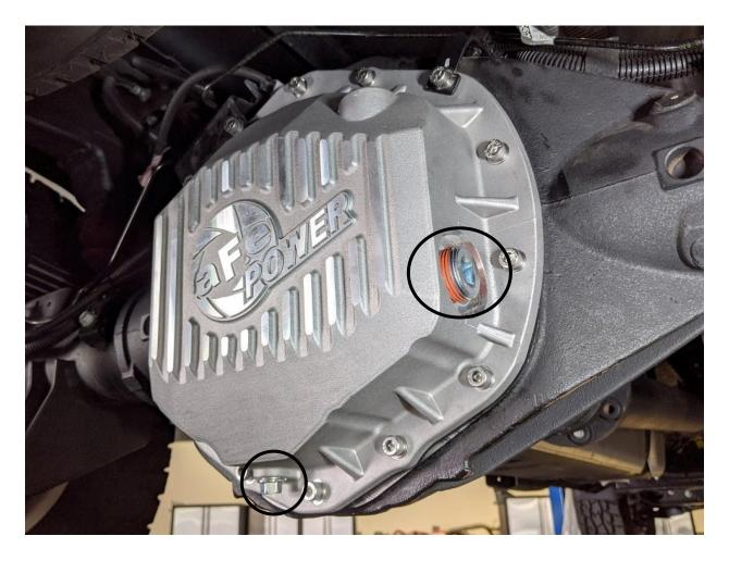
20. Install the supplied M12x1.25 drain plug and crush washer into the bottom of the cover.
