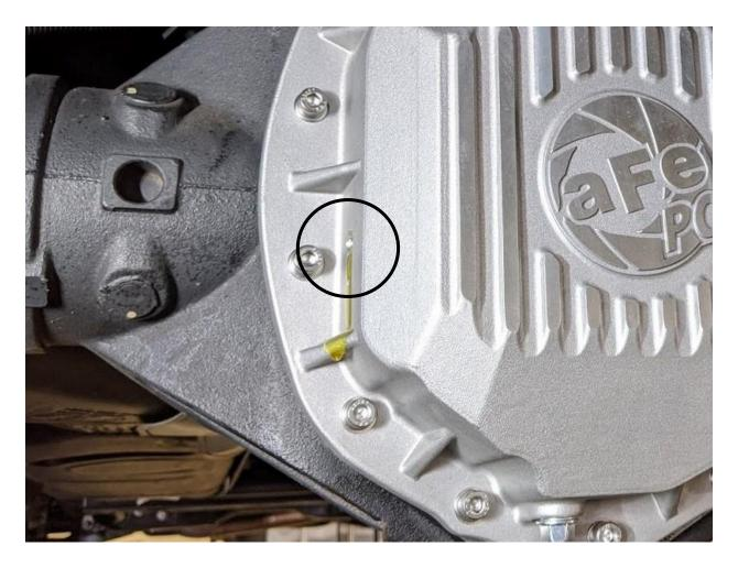
Note: Place a drain pan under the differential cover before refilling.
