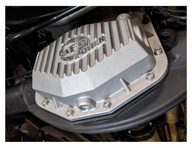
17. Install the supplied M12x1.25 drain plug and crush washer into the bottom of the cover (secure about  $\frac{1}{2}$  turn past finger tight).
