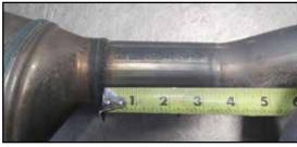
Step 9: Now cut with a hack saw at your mark as straight as possible and deburr when complete.
