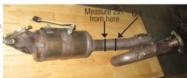
Note: aFe recommends that the tailpipe be at least 1/2"-1" away from any body panels to avoid heat related body damage. Tighten and secure.
