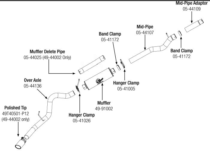
**Step 1: (Read Instructions prior to installation)** Remove your stock exhaust up to the cataytic converter from the rear of your truck working your way forward. It may be necessary to cut the pipes if the slip joints are stuck. Take caution not to damage the factory isolation mounts as they will be reused.
