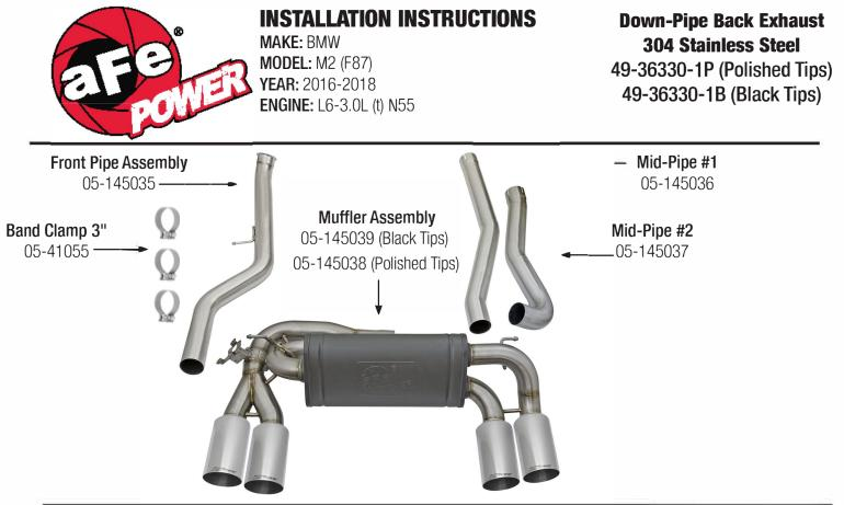
Professional installation is highly recommended. (Read instructions prior to installation). Make sure to always have at least (2) stands or jacks on hand to support the removal of OE system. Also for the installation of aFe system. Any Removal of rubber isolation mounts may require using a spray lubricant such as WD40 and a pry bar.
