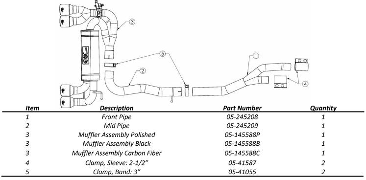
**aFe POWER recommends professional installation on this product.** Thoroughly inspect the aFe POWER exhaust system to make sure there is no damage from shipping (if damage is noted, immediately contact aFe POWER customer service). Allow time for your vehicle to cool down prior to installation. When working on your vehicle proceed with caution. Wear protective safety equipment; eye goggles and gloves to ensure a safe installation.
