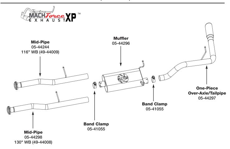
Step 1: (Read Instructions prior to installation) Remove your stock exhaust up to the catalytic converter from the rear of your truck working your way forward. Take caution not to damage the factory isolation mounts as they will be reused. This system is best installed with a chassis lift with axles extended for clearance. It is recommended to not fully tighten the clamps until the entire system has been installed.
